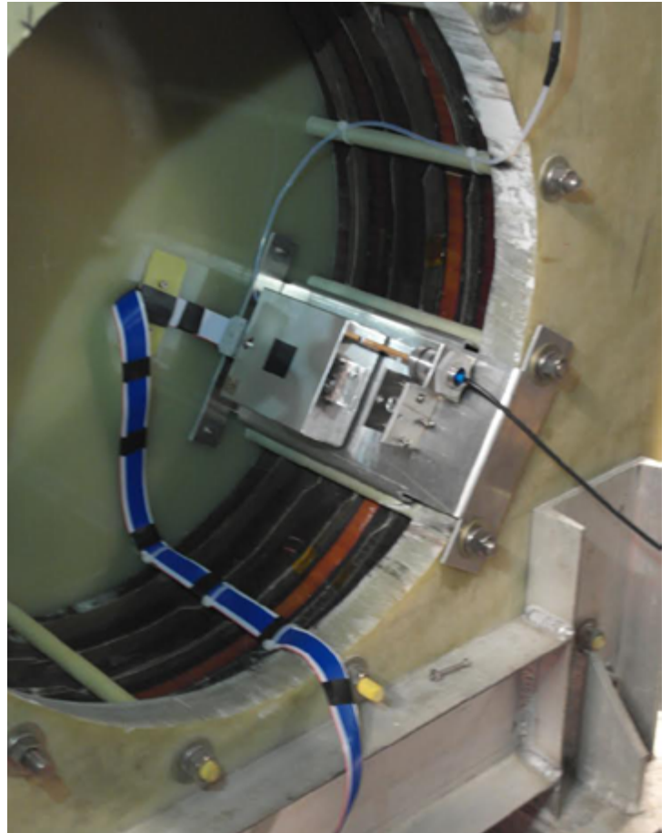
The spectrometer mounted in the bore of the coils. (Photo by John Greenwald)
