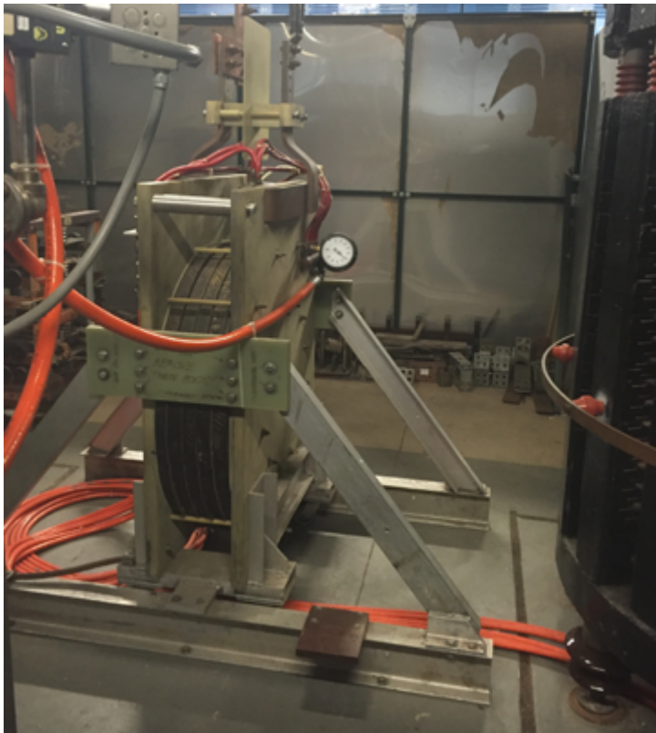
The dummy load before technicians cut an opening into the support plate. (Photo by Charles Neumeyer)
