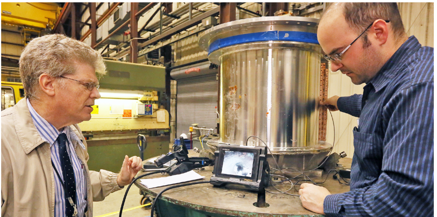
Engineers Irving Zatz, left, and Joseph Petrella perform tests on the PF1A upper coil during a forensic investigation last fall. (Photo by Elle Starkman)
