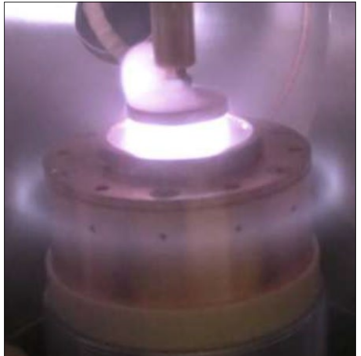
Laboratory test of a liquid-metal cathode.
