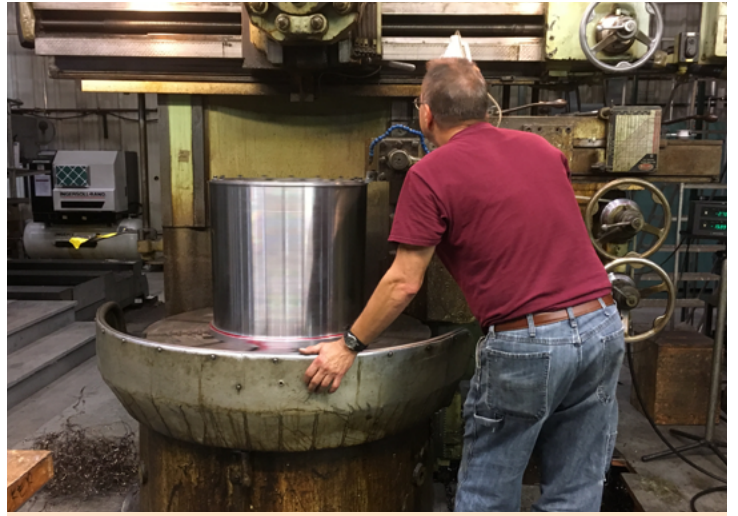
A technician examines the winding mandrel. (Photo by Richard Burke)
