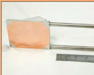
3D printing, bottom left: completed stainless steel and copper mirror system; top left: completed mirror system with initial version of the stainless steel part; right: Bob Ellis with a 3D-printed plastic prototype for another part of the launcher.
