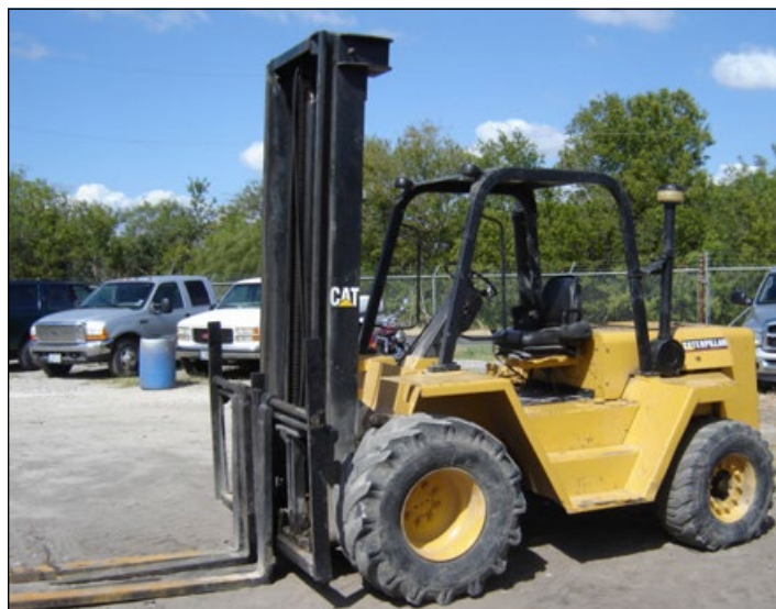
Operators of large machines like the forklift shown here must now inspect the equipment and fill out an operator's daily checklist or ODCL before operating machinery. (Stock photo).
