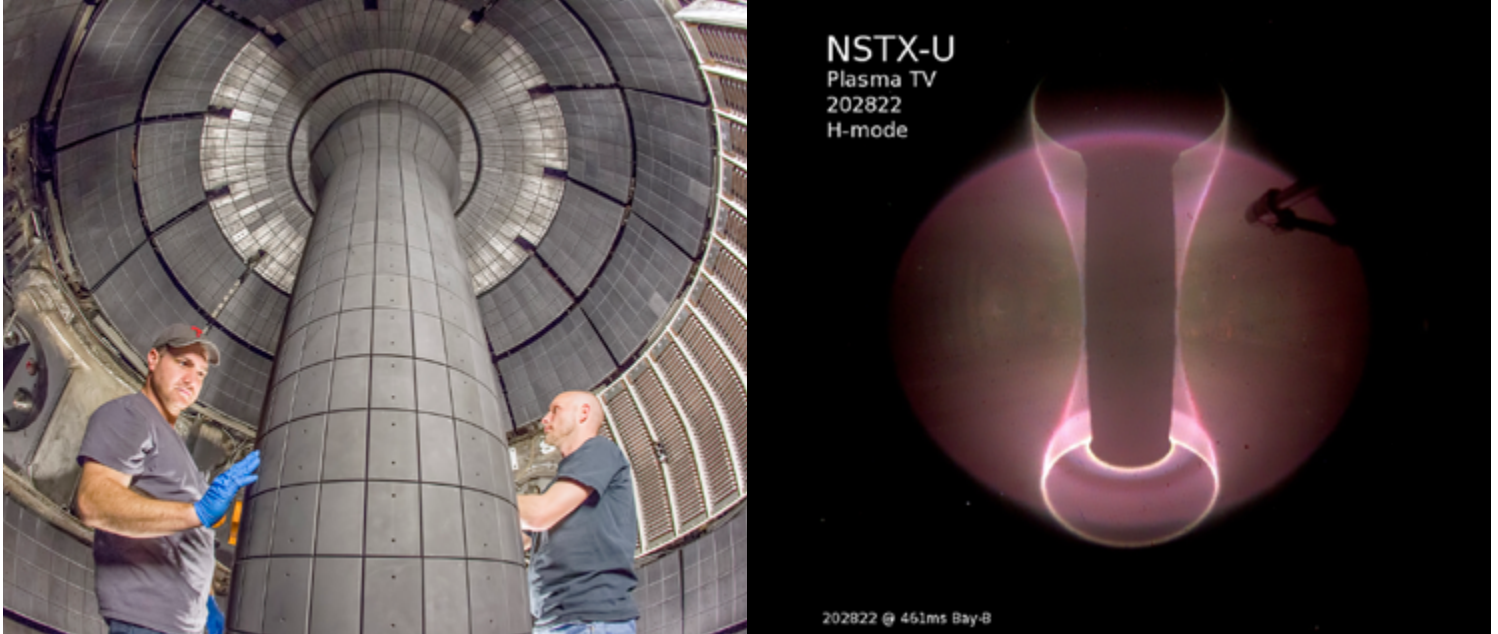
The new NSTX-U center stack central magnet that doubles the magnetic field and plasma current, left, and an image of NSTX-U H-mode plasma. (Photo by Elle Starkman/PPPL Office of Communications. Right: NSTX-U Team)
