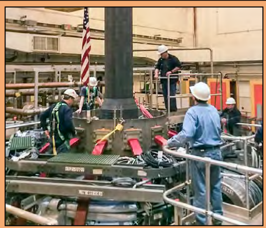
Technicians guide the center stack into the vacuum vessel.
