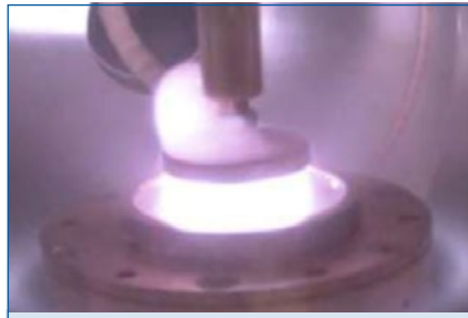
Laboratory test of a liquid-metal cathode (Courtesy of General Electric.)
