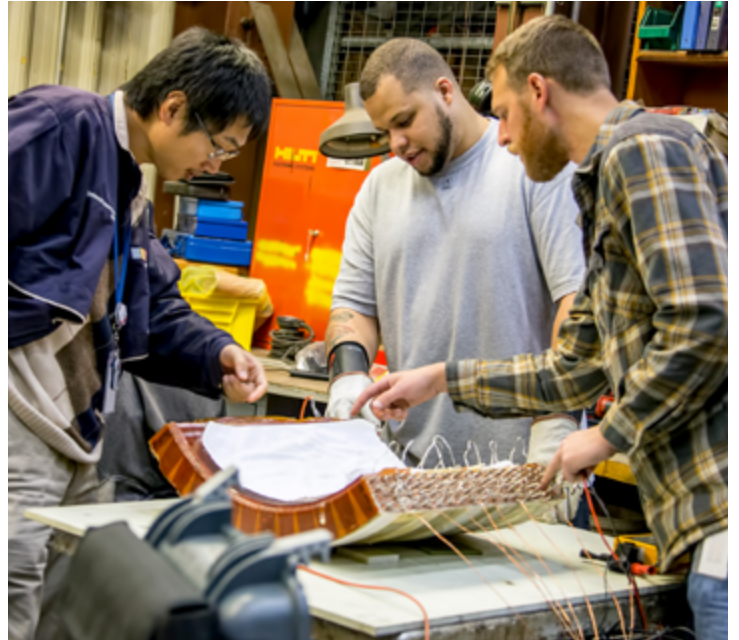
Engineer Weiguo Que, left, and technicians Alexis Sanchez, middle, and Elliot Baer, perform electrical tests on a segment of the coil. (Photo by Elle Starkman)
