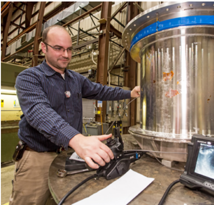
Engineer Joseph Petrella, who supervised the tests, uses a borescope to capture an image of the interior of the coil. (Photo by Elle Starkman)
