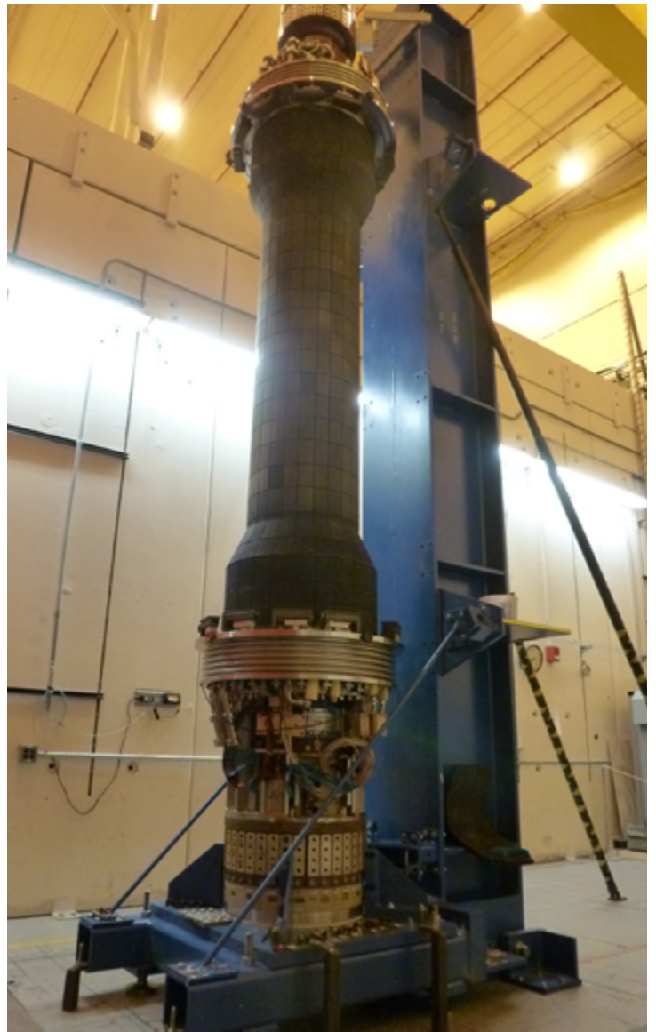
The NSTX-U center stack in the D-Site south high bay. (Photo by Erik Perry)
