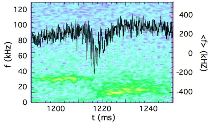
Figure 3. Frequency of Mirnov coil signal (left axis) and Doppler peak (right) for a dynamic configuration scan during the time at which the 5/3 resonance passes through the reflecting layer.
