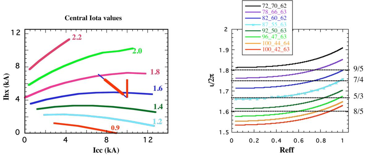
Figure 1. Left: configuration diagram of the TJ-II with central  $\iota$  values as a function of the currents in the central conductors. Two line segments are examples of performed configuration scans. Right:  $\iota$ -profiles in a configuration scan.
