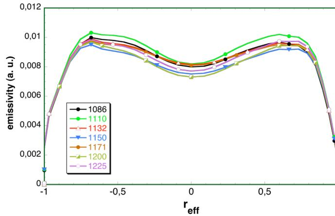
Figure 4. Reconstructed emissivity profiles from bolometer arrays during a dynamic scan discharge that makes the 5/3 and 7/4 resonances cross entirely the plasma during the times shown.
