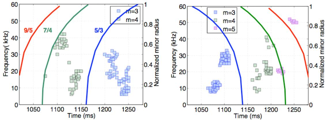
Figure 2. Frequencies and mode numbers resolved by the array of Mirnov coils in two dynamic configuration scans: downward (left) and upward sweeping (right).
