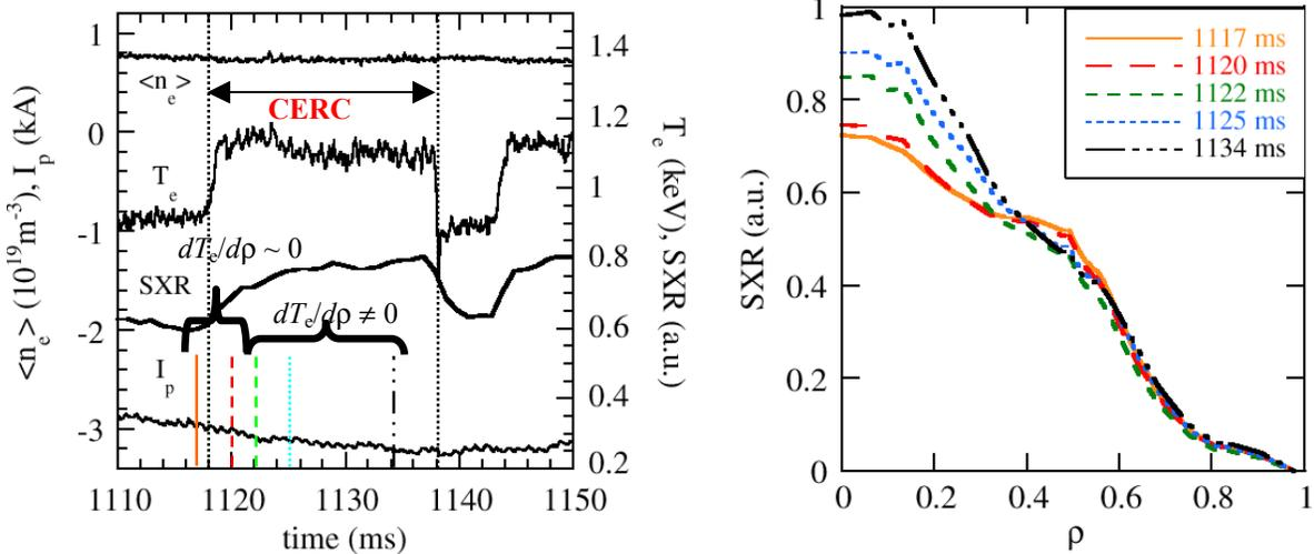
Fig.5 Time evolution of electron density, electron temperature, SXR and plasma current in CERC formation (Left). SXR profiles (Right) [14].
