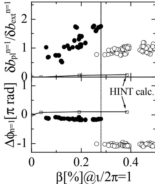
Fig.3 Dependence of resonant field amplitude (upper) and difference of toroidal angle on beta
