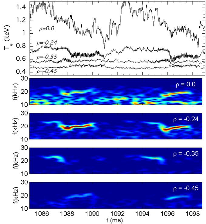
Fig.6 Time evolution of electron temperature (Upper) and spectrum of ECE (Lower) [16]. CERC is formed from  $t = 1092$ [ms] to  $t = 1096$ [ms].
