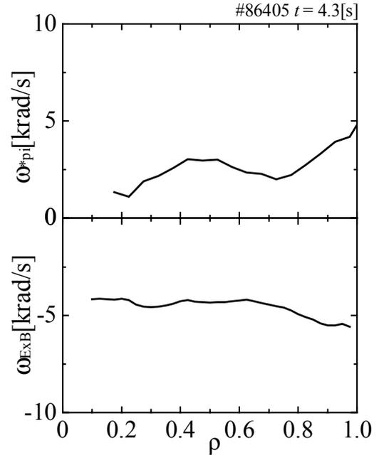
Fig.7 Minor radius profile of ion diamagnetic angular velocity  $\omega_{*pi}$  (a) and  $E \times B$  drift angular velocity  $\omega_{E \times B}$  (b).
