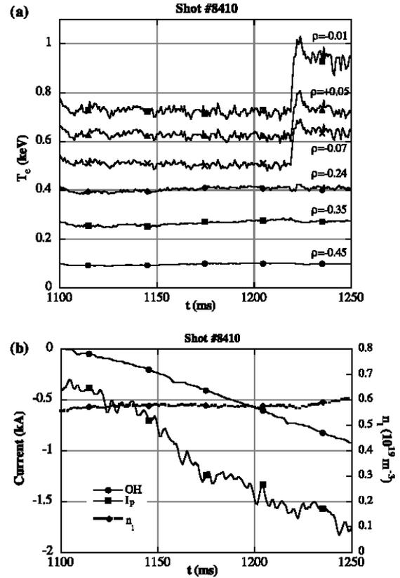
Fig.4 Time evolution of (a) temperature and (b) line density, OH coil current and plasma current for the case of Ohmic current induction [6].
