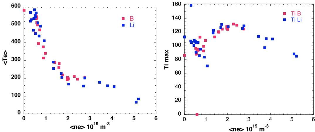
Figure 1. Evolution of average plasma electron (left) and ion (right) temperature with electron density for B and Li coatings.
