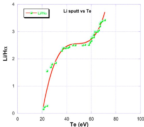
Figure 6. Li sputtering yield (a.u.) versus electron temperature at  $r=0.95$
