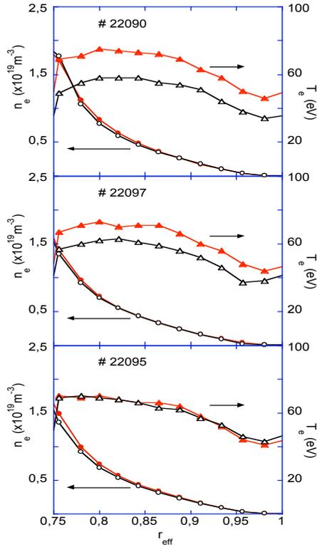
Fig.5 Edge profiles of electron density and temperature before (red lines) and after (black) Ne-seeded H<sub>2</sub> injections.
