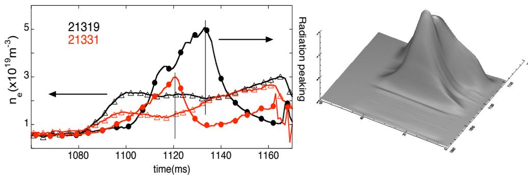
Figure 4. Left) Time stories of electron density and radiation peaking factor for two shots with forced (#21331) and spontaneous (#21319) bell-dome transition. Right) time evolution of emissivity profiles showing the changes from peaked to dome profiles (shot #21319).
