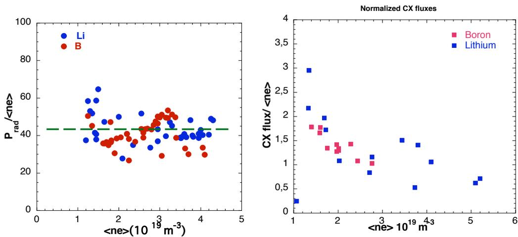
Figure 2. Normalized radiation (left) and CX (right) losses for B and Li coatings
