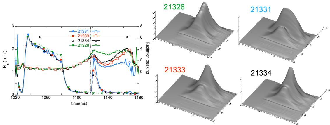
Figure 3. Induction of profile transition by a short gas puff at different amplitudes. For very low levels (21333 and 34) a reversible transition back to the bell type profile is seen. Full emissivity profiles are shown at the right for each discharge.
