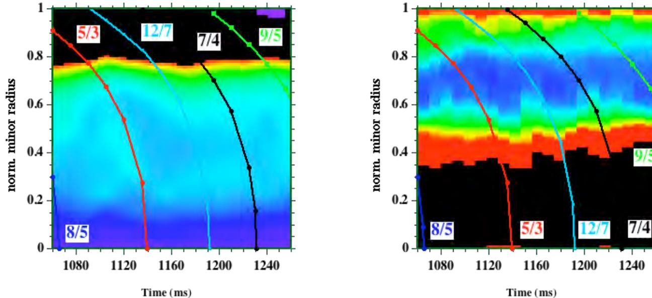
Electron temperature and density gradients (respectively obtained from ECE and reflectometry data) yield effective diffusivities that seem to move likewise through the plasma. Taking the paths of the resonances as a guide, ridges of  $\chi_e$  and  $D_e$  follow the same lines.
