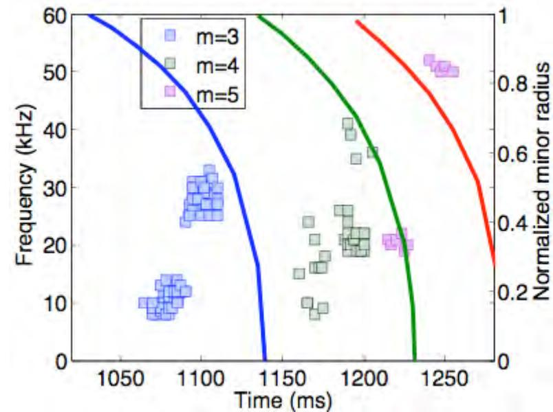
As the feeding currents in the central (circular and helical) conductors of the device are ramped in time, **magnetic resonances move through the plasma**. Mirnov coil arrays allow for obtaining **mode numbers** and associated **frequencies**. The lines represent the location of vacuum resonances 9/5, 7/4 and 5/3.
