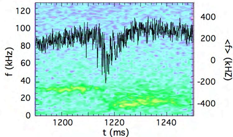
Displacement of the main frequency of the density fluctuations at fixed radial position ( $\rho \approx 0.8$ ) and mode frequency from magnetics at the passage of a resonance.
