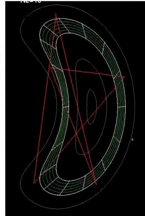
**3-D ion velocity distribution** obtained from the ion distribution function (left). The geometry of the TJ-II has been straightened (center) for clarity, where we can see the alignment of magnetic field lines –green– and calculation mesh –white. The results correspond to the plasma corona shown (right), which includes the  $8/5$  vacuum resonance
