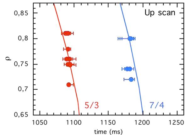
Radial (norm. flux surface coordinate) position of the vacuum resonances 7/4 and 5/3 and time laps during which a differential rotation is detected in the indicated radial positions. Data correspond to downwards (left) and upwards (right) moving rotational transform.
