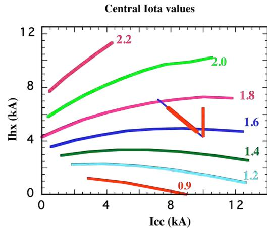
With proper combinations of  $I_{hx}$  and  $I_{cc}$ , the configuration map can be scanned
