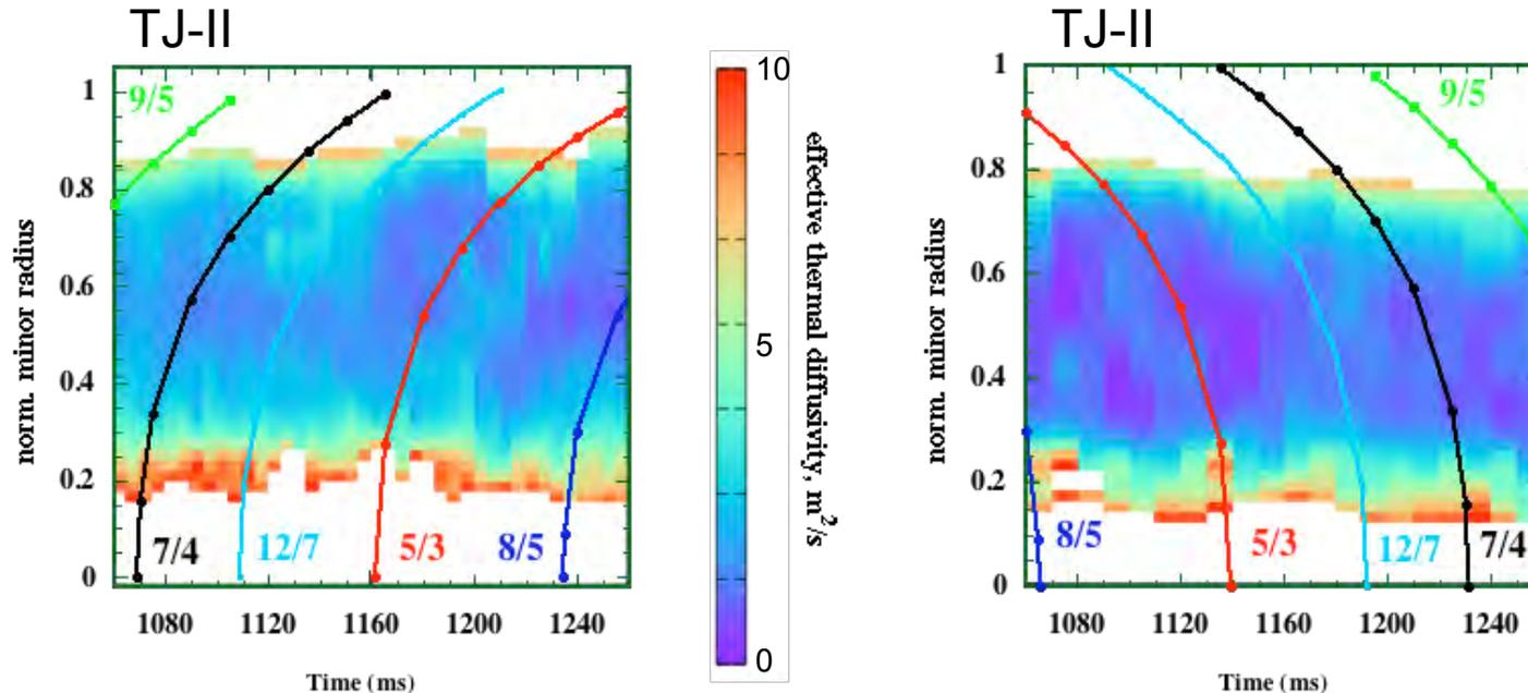
Same pattern as in static configuration scans but now found dynamically (single discharge sweeping). There is absolutely no doubt, after many experiments of this kind, that the furrows and ridges in  $\chi_e$  are lines of iso-“rotational transform”. Very important:
