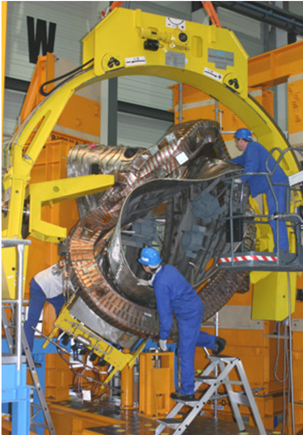
Coils are threaded across the plasma vessel
