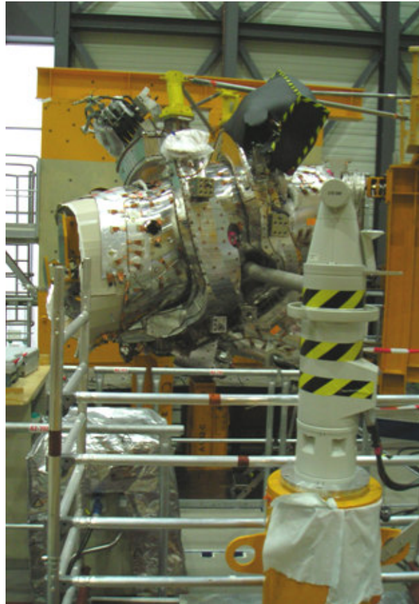
Thermal insulation is completed
