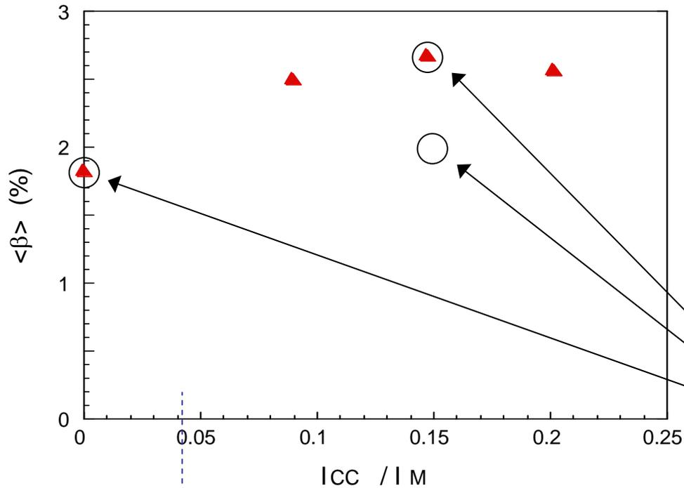
*Variation of peak- $\langle \beta \rangle$  versus the divertor control-coil current  $I_{CC}$  normalized by the modular coil current, for  $B=1.25$  T,  $P_{NB} = 2.8$  MW absorbed and  $\iota_{vac} = 0.44$ .*
