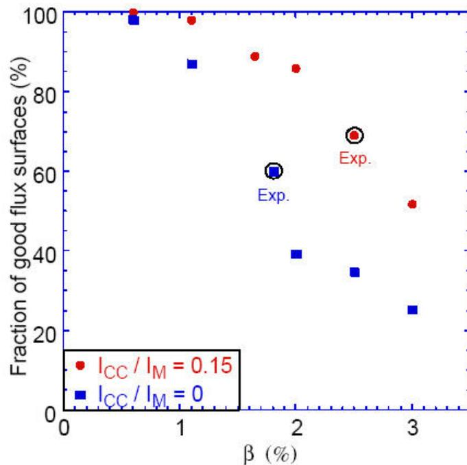
Fraction of good flux surfaces versus  $\beta$  as predicted by PIES for two different values of the control coil current for the W7AS stellarator. The circles indicate the PIES calculations done for the experimentally achieved value of  $\beta$ .
