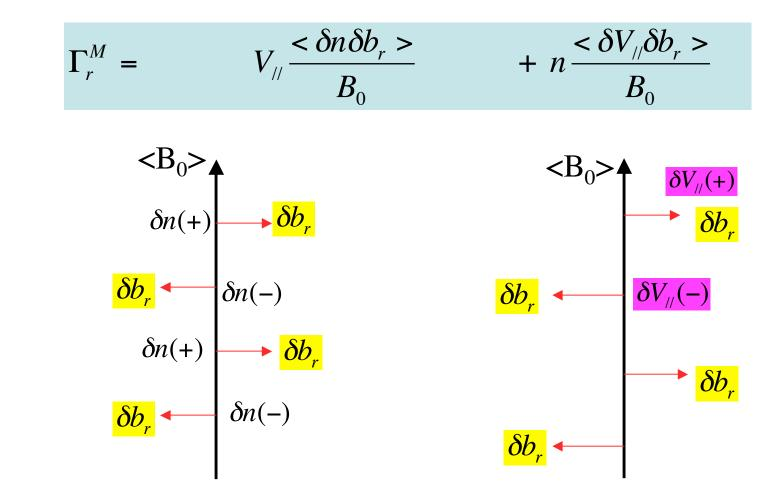
Density-fluctuation dependent flux Velocity-fluctuation dependent flux Measurement of Magnetic Fluctuation-Induced Particle Flux
