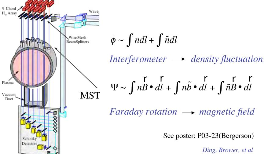
11 chords, separation 8 cm, phase resolution 0.05 degree, time response up to 1 µs
