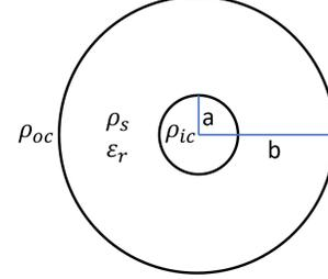
Fig. 3. Lumped-element in the Transmission Line Model
