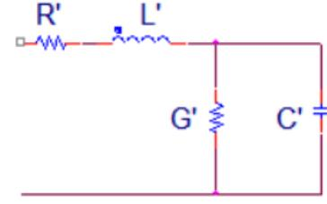
Fig. 2. Lumped-element in the Transmission Line Model
