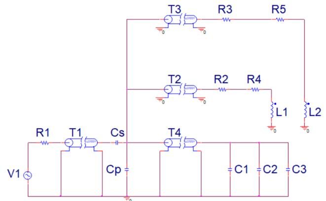
Fig. 1. PSpice schematic of the PFRC's RF system
