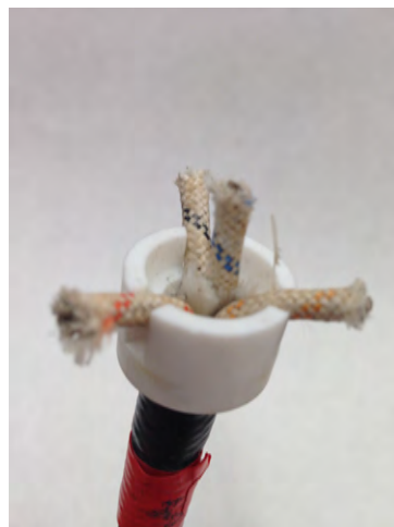
(b) Cable with Macor Housing
