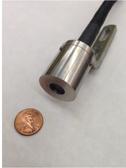
Figure 3: Final Assembled RPA (Penny for Scale)
