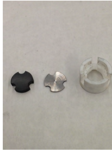
(b) Graphite Detector with Conductor Lead and Macor Housing
