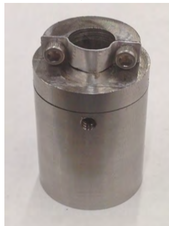
(d) Assembled Stainless Steel Housing and Cap
