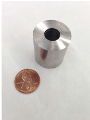
(a) Stainless Steel Housing Viewed from Sensing End (Penny for Scale)
