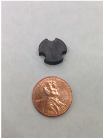
(a) Graphite Detector (Penny for Scale)
