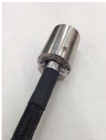
(a) Fully Assembled RPA Showing the Cable Entering the Back
