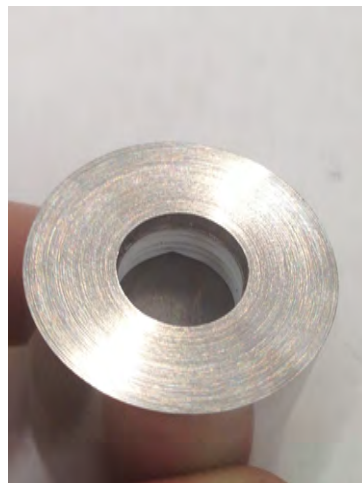
(d) Assembled Washers, Detector, and Macor Housing to Show Operational Area of RPA (Minus the Grids)
