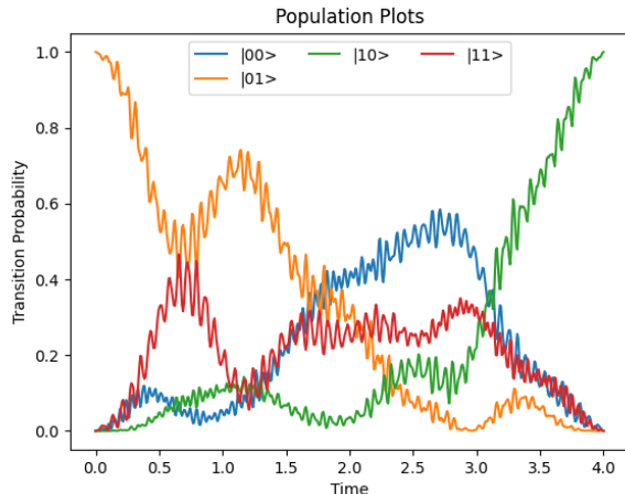
FIG. 9: Populations of all four computational basis states described by Eqs. 17 and 18 under the effect of the SWAP gate acting on |01\rangle .
