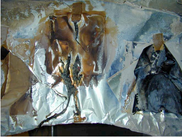
Figure 3: Plastic film samples after exposure to Lithium plasma
