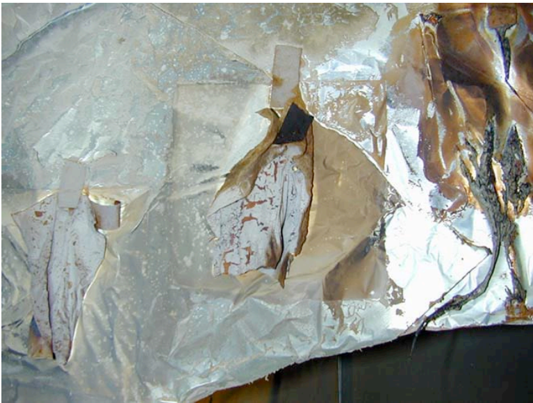
Figure 4: More Plastic film samples after exposure to Lithium plasma
