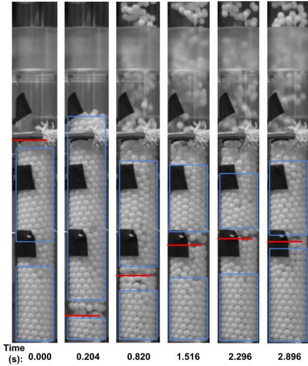
Figure 13: This figure shows the initial height progression of where bed separation occurs. Additionally the conical formation of the outer layer is shown. This occurred with the bottom mesh set up with a starting bed height of 18.5 cm and an inlet velocity of 0.397 m/s.
