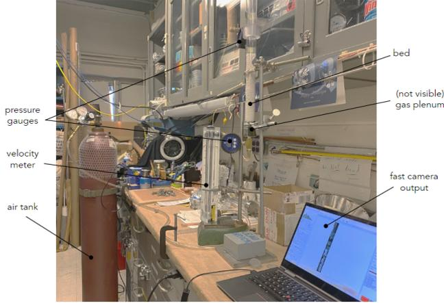
Figure 5: The experimental single-cylinder configuration above has a 24 cm starting bed height with the bottom mesh setup. Two pressure gauges are shown, each an SSI Technologies, LLC digital gauge with an accuracy of  $\pm 0.001$  psi, the first is located just below the inlet and the second is located 6 cm above the starting bed height at a height of 30 cm.
