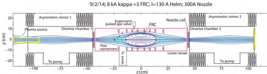
FIG. 1: A) View of the PFRC-2 in capacitively coupled mode. B) View of the PFRC-2 in field-reversed configuration.
