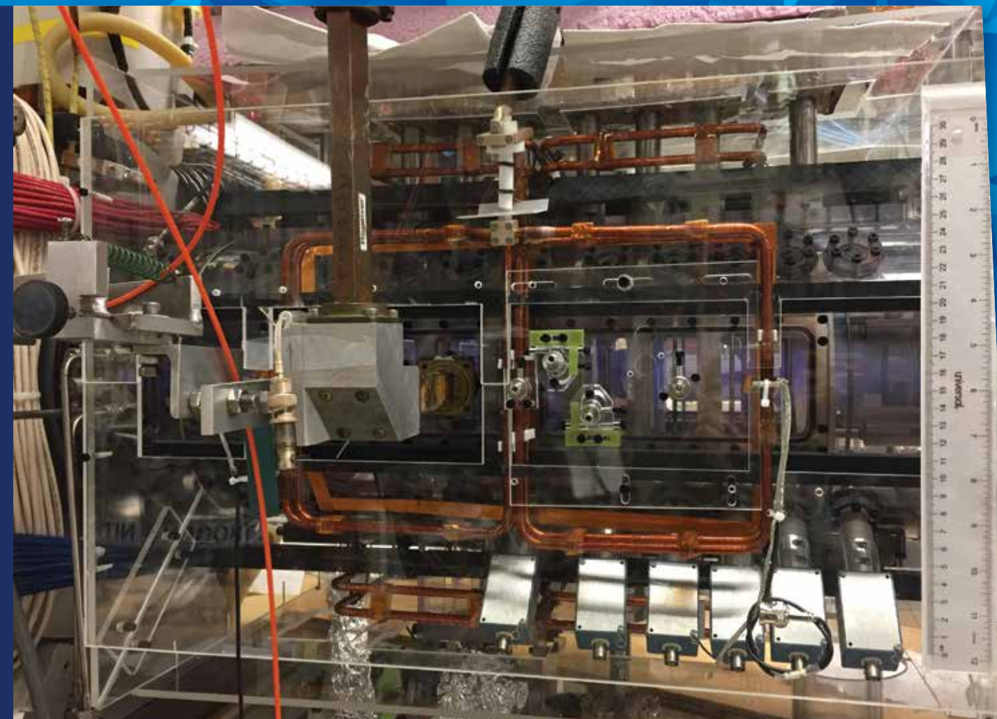
A DFD prototype. The copper-colored RF-heating antennas can be clearly seen.
