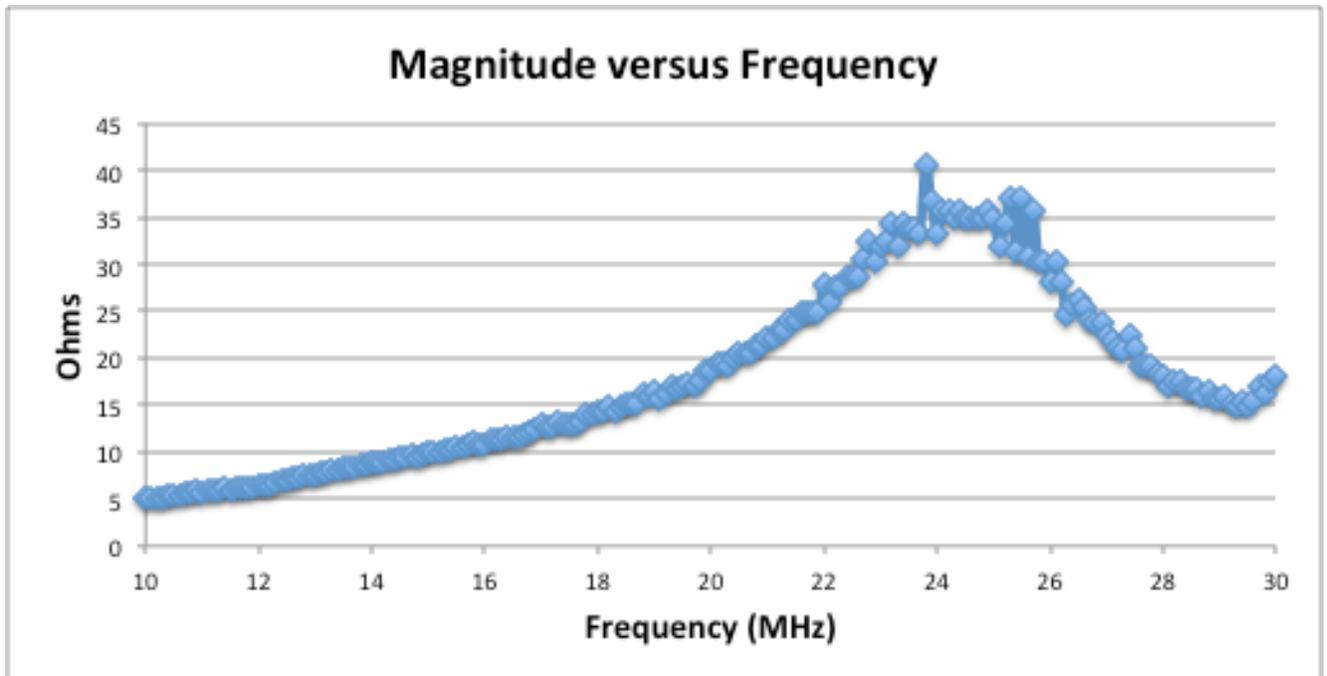
This is a graph of the resistance of the antenna versus the applied voltage frequency. One can see a clear spike at around 25MHz, where the antenna is at resonance. In order to be matched, the antenna must stay on the low end of the resonance spike, which ruled out using a higher frequency of 27MHz instead of 13.56MHz.
