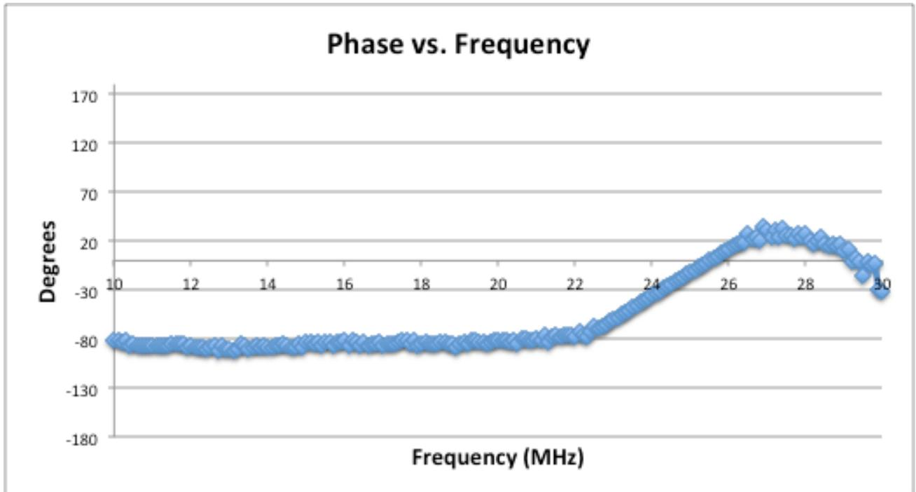
This graph shows the phase of the impedance as a function of the frequency- note that it crosses from negative to positive at resonance.
