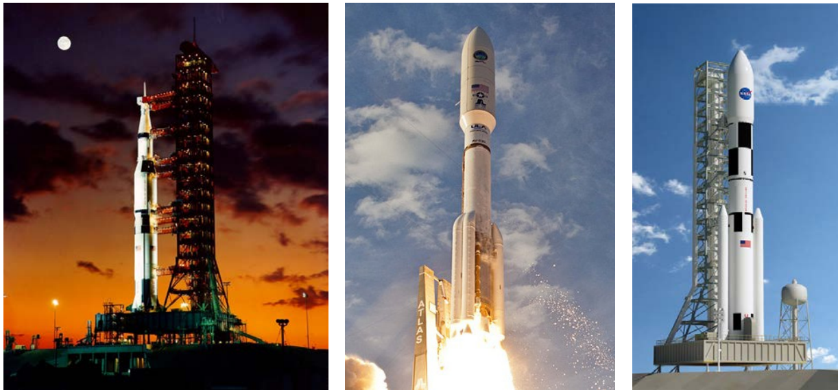
Figure 3. (Credit NASA). Examples of the best heavy lift chemical rockets: Saturn V launch vehicle sitting on the pad (left), with third stage J2 engine specific impulse of 420 seconds, and thrust of 1,000 kN. New Horizons Pluto mission at launch on an Atlas V rocket (middle). NASA's new Space Launch Systems heavy launch vehicle (right).
