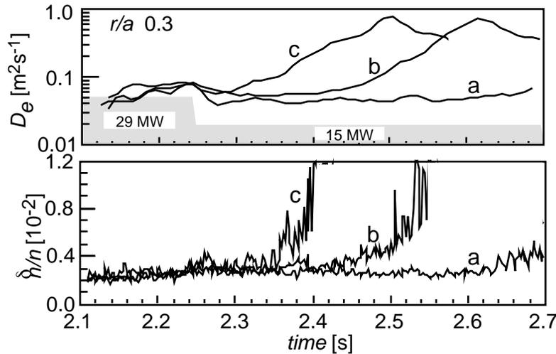
FIG. 6. Electron particle diffusivity and amplitude of density fluctuations at  $r/a = 0.3$ ; a - balanced injection, b - co/counter=5/1, c - co/counter=6/0.
