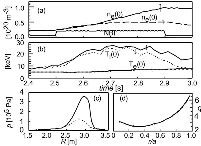
FIG. 1. Time evolution of central electron density (a) and temperatures (b) in ERS (solid line) and RS (dashed line) plasmas with 29 and 27 MW of balanced NBI, respectively. The bottom graphs show the radial profile of the plasma pressure (c) at  $t=2.9$  s. and the safety factor (d) at the bifurcation time.
