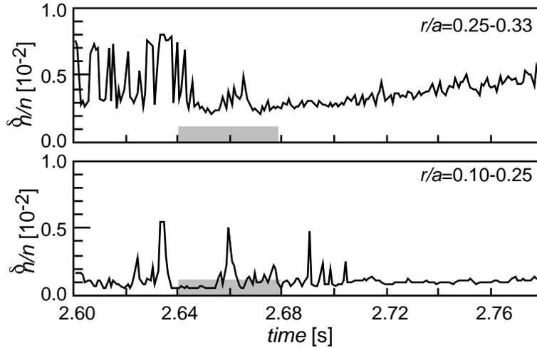
FIG. 3. Time evolution of density fluctuations in the ERS mode. The shaded area represents the time of bifurcation.
