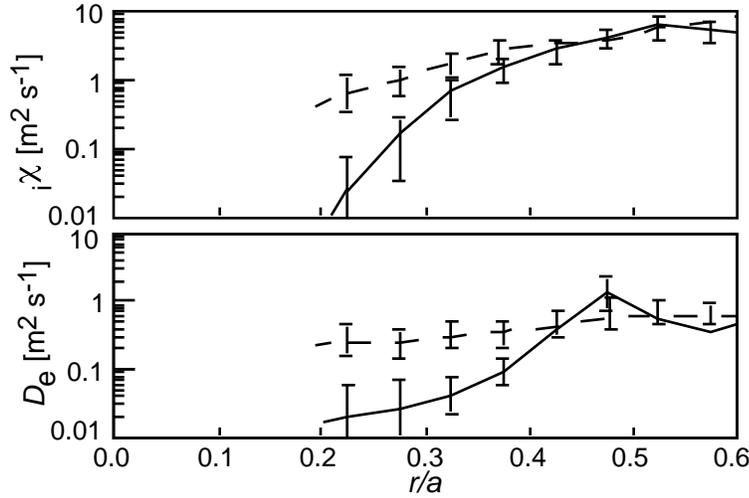
FIG. 2. Electron particle diffusivity ( $D_e$ ) and ion thermal conductivity ( $\chi_i$ ) in the ERS (solid line) and RS (dashed line) plasmas of Fig. 1 ( $t=2.75$  s).
