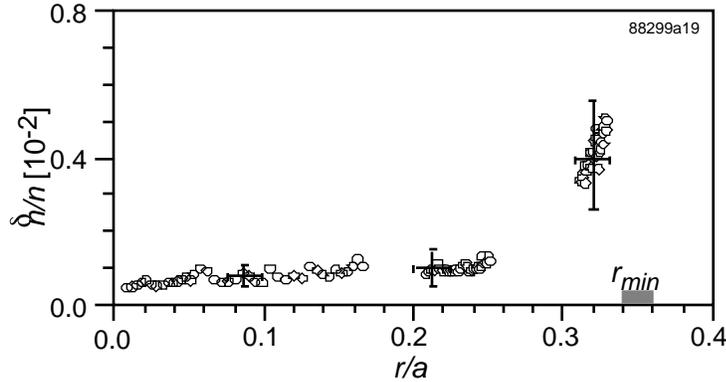
FIG. 4. Amplitude of density fluctuations in the ERS mode of Fig. 1 at  $t=2.72-2.78$  s;  $r_{min}$  is the radial position with minimum  $q$ .
