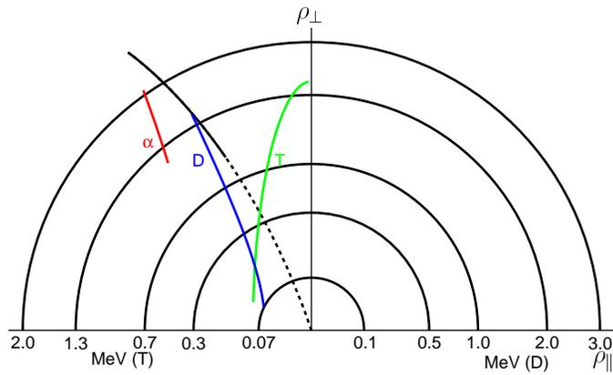
Fig. 3: Passing/trapped boundary and trajectories of 100 keV D, 100 keV T and 3.5 MeV  $\alpha$  particles diffused by IBW vs.  $\rho_\parallel$  and  $\rho_\perp$ .
