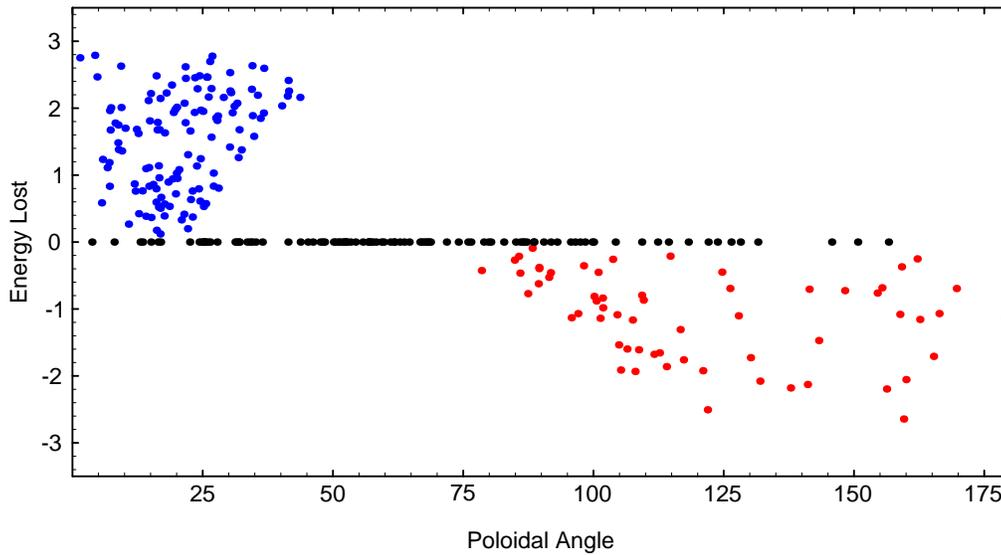
Fig. 6: Energy lost to the wave (MeV) and poloidal exit angle of  $\alpha$  particles in simulated reverse shear TFTR discharge with  $B = 5.3$  T,  $I = 1.85$  MA (scaled shot #84011). 1000 particles are simulated. Particles exiting with zero energy lost correspond to first orbit losses (11%). 13.7% of the  $\alpha$  particles are cooled, exiting near the outer midplane. 3.8% are heated exiting between the inner midplane and the bottom.
