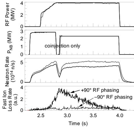
Fig. 4 Losses of co deuterium beams in the presence of phased rf.  $+90^\circ$  phasing (counter to the current) results in significantly enhanced losses, whereas  $-90^\circ$  phasing (co to the current) shows first orbit losses of fusion products only.
