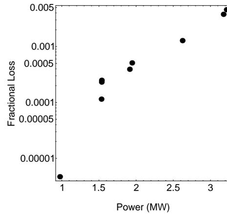
Fig. 5 Approximate losses of deuterium ions (fraction of beam ions) vs. rf power. The measured loss is assumed to be constant over a portion of the outer midplane.
