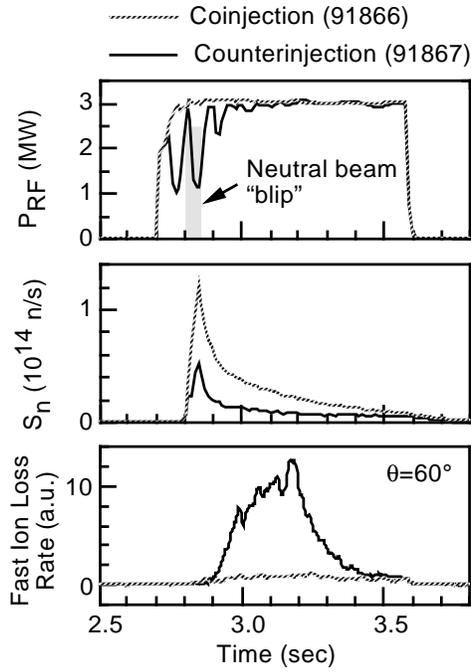
Fig. 1 Losses of co and counter deuterium beam ions in the presence of  $\pi$  phased rf. Discharge at 4.8 T, 1.4 MA with mode conversion layer on axis.
