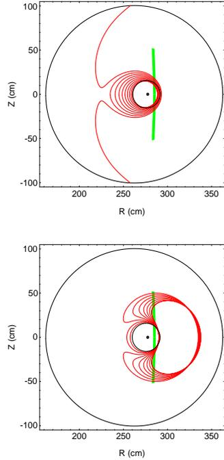
Fig. 2 A deuteron (top) and a triton (bottom) interacting with an IBW (shaded strip). The 100 keV particles are initially passing near the center, later becoming trapped.
