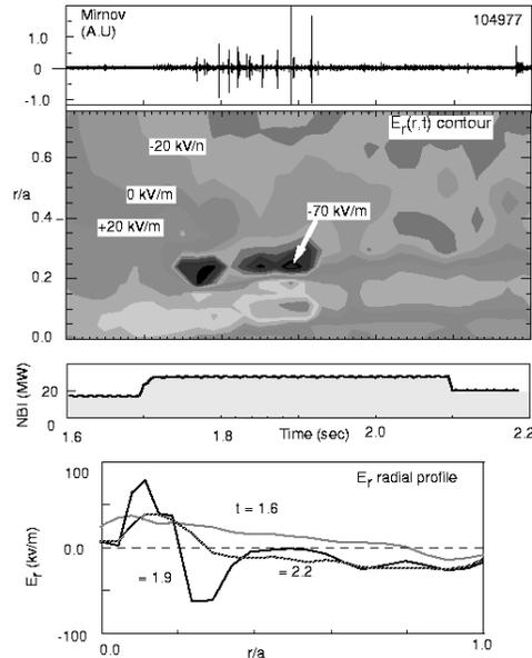
Figure 3: The BLM activity in TFTR sometimes coincides with intense negative radial electric fields. The top trace shows the Mirnov signal, the middle panel shows contours of the radial electric field which changes with time. The radial profile of  $E_r$  at times corresponding to the BLMs is shown in the lowest panel. Note that while the field shown here has a maximum negative value of  $60\text{kV/m}$ ; in some bursts, field strengths in excess of  $100\text{kV/m}$  have been observed.
