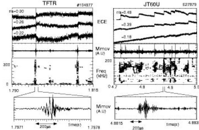
Figure 2: Traces of  $T_e$  and the Mirnov activity on TFTR and JT-60U showing the similar burst-like features of BLMs in both devices. Note the spatial localization and inversion in the  $T_e$  traces. The Mirnov activity coincides with the  $T_e$  bursts and the mode is seen to grow on a time scale shorter than  $100\mu s$ .
