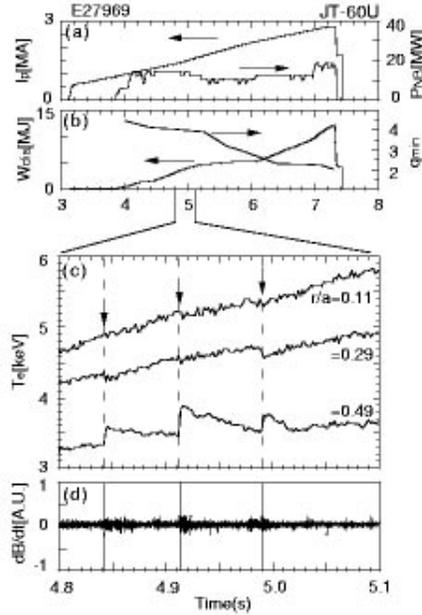
Figure 1: Time evolution of the (a) plasma current,  $I_p$ , neutral beam injection power  $P_{NB}$ , (b) stored energy,  $W_{dia}$ , and  $q_{min}$  on JT-60U for the length of the discharge. Panels (c) and (d) show an expanded view of a shorter time segment, where (c) has the evolution of  $T_e$  at three radii, and (d) shows the data from a Mirnov loop. Note the spatial localization and inversion in the  $T_e$  traces. The Mirnov activity coincides with the  $T_e$  bursts.
