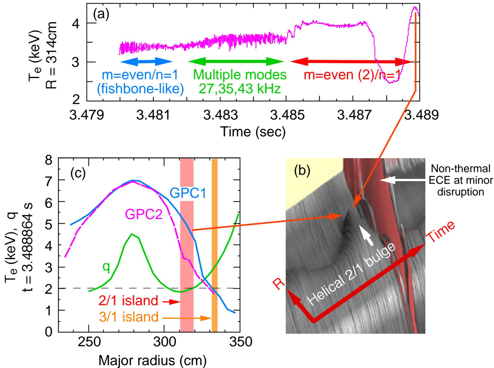
Fig. 3 Helical snake in the island X-point near  $q_{\min}$  before minor disruption.  $q$ -profile from TRANSP
