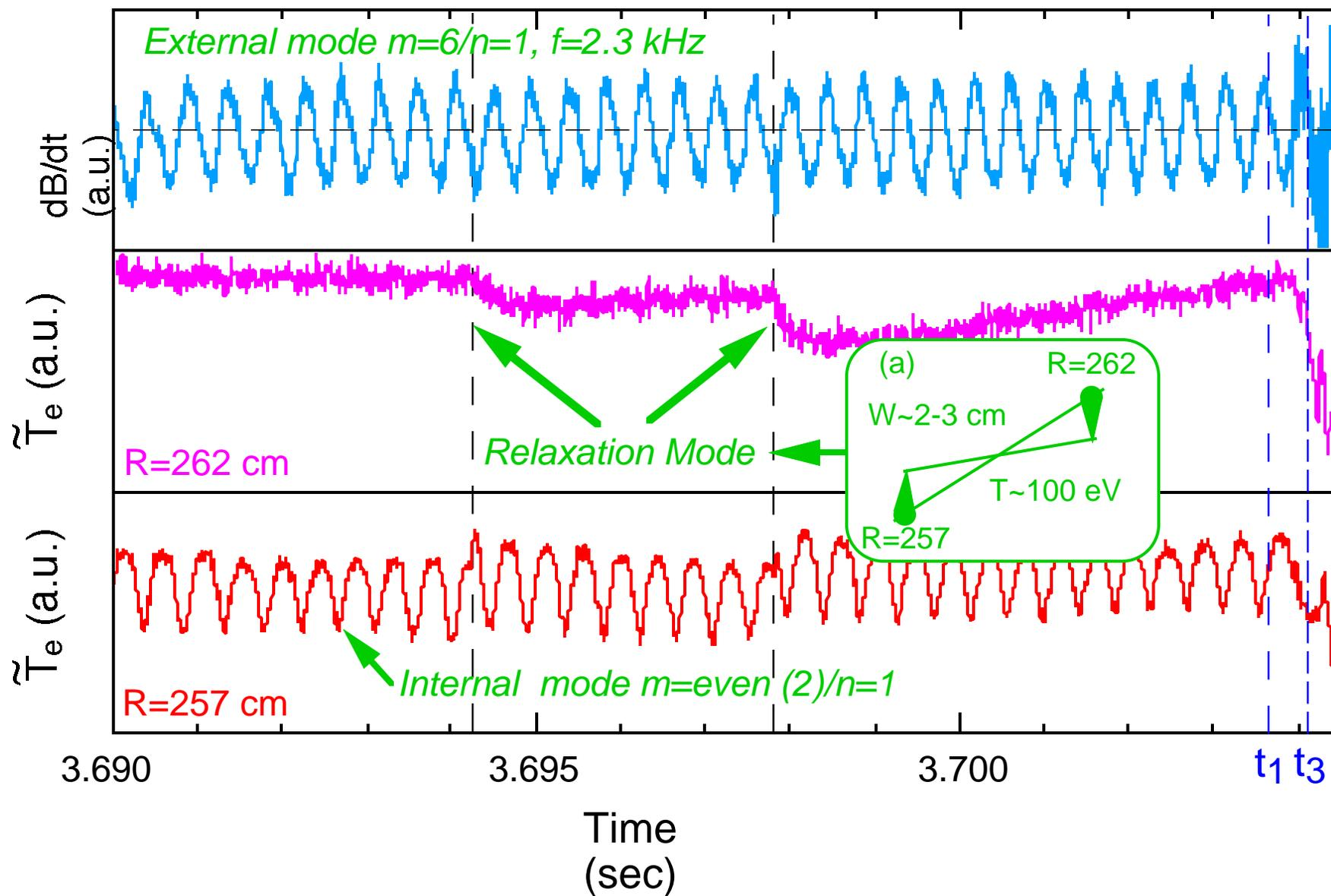
Fig. 2 Relaxation phenomena in the border between negative shear region and  $q_{\min}$  prior to disruption
