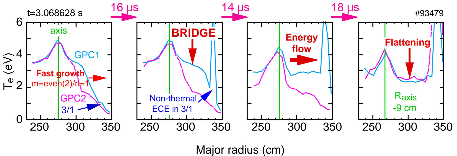
Fig. 4 Development of localized "bridge" between core and edge causes rapid cooling of center and inward shift of axis
