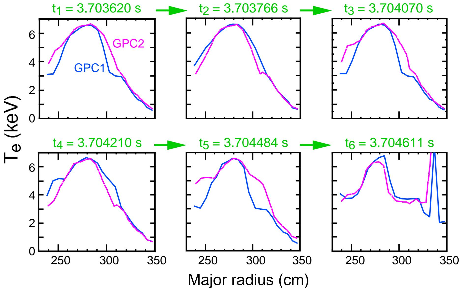
Fig. 1a Sequence of temperature profiles during a disruption in a RS plasma. Toroidal locations separated by  $126^\circ$ .
