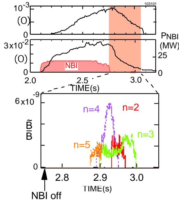
Fig. 5. Time evolution of  $\beta(0)$  and  $\beta(0)$  and Mirnov coil data showing TAE signatures.
