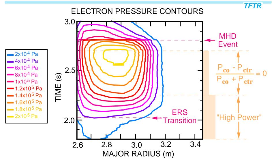
Steep electron pressure gradient at R ~ 3.05 m persists throughout balanced injection postlude.
