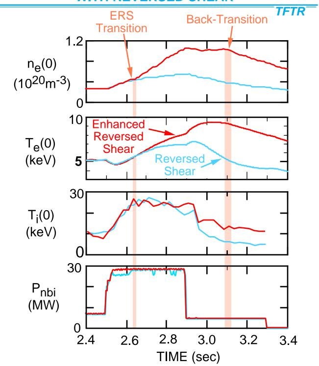
Abrupt transition to reduced particle and thermal transport in Enhanced Reversed Shear (ERS) discharge.
