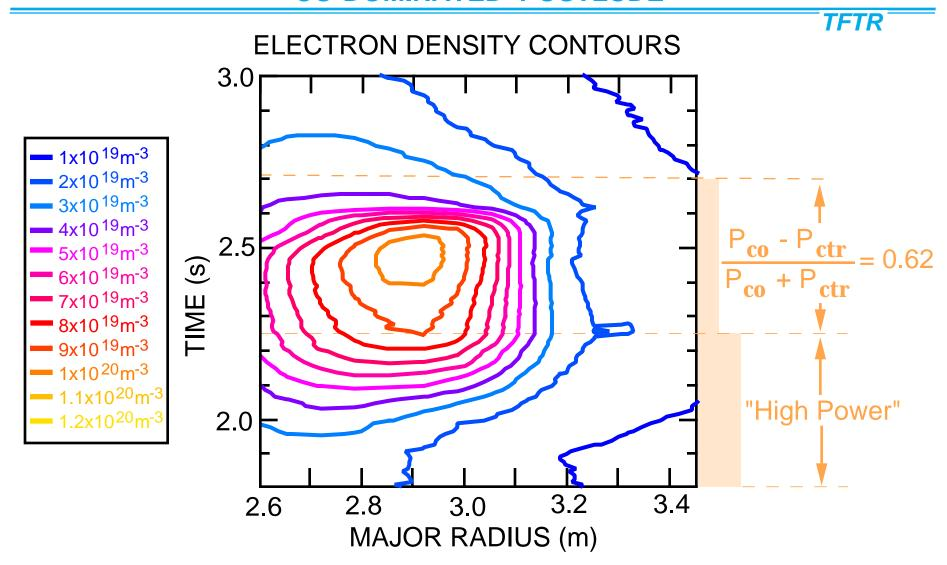
Electron density degrades before electron temperature during co-dominated postlude.
