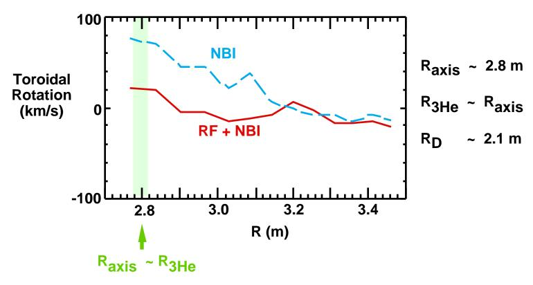
no core (r/a 0.5) beam - rf resonance but reduction effect remains
