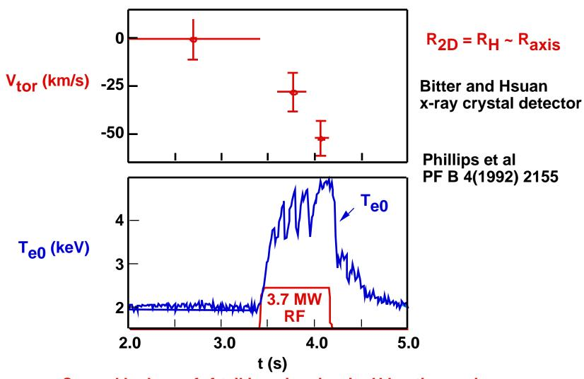
Caused by loss of rf-tail ions in minority H heating regime
