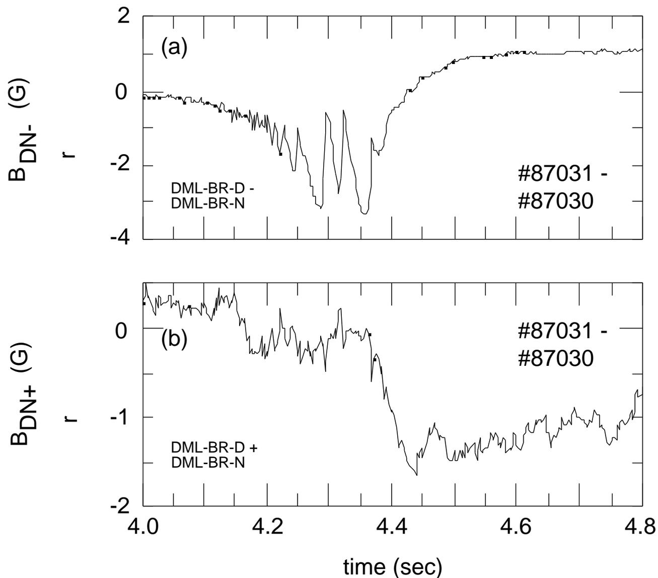
**Fig. 6** Both difference and sum of SMP signals from a toroidally opposite sensor pair are examined. The sum and difference signals contain a *secularly* growing component. The difference signal contains also a slow oscillating component. The secular component *cannot* be produced by MHD modes alone. The SMP signal must have contributions from an additional source.
