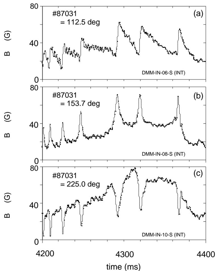
**Fig. 13** Waveforms of Mirnov signals show strongly distorted time coherence at all poloidal locations.
