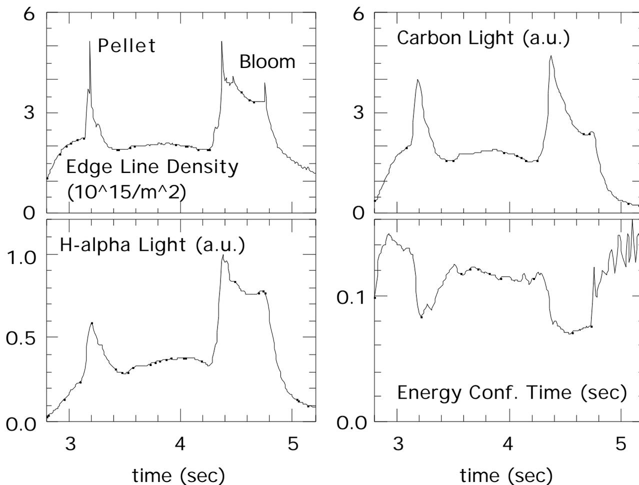
**Fig. 3** In a 'bloom' light emission increases from hydrogenic atoms and carbon impurity ions. Density increases first at edge. Energy confinement degrades. (The peak at 3.2 sec is an unrelated Li-pellet injection.)
