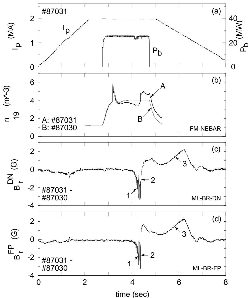
**Fig. 1** An overview of discharges with SMP and 'bloom' events (see below for details). (a) Two discharges had identical  $I_p$  and  $P_b$  waveforms. (b) In Discharge A, an edge event, termed 'bloom' in TFTR lingo, took place around 4.2 sec when density rose strongly. (An earlier density peak was caused by unrelated Li-pellet injection.) In Discharge B, no bloom occurred. (c) and (d) An SMP event at '1' and '2' occurred concurrently with bloom.
