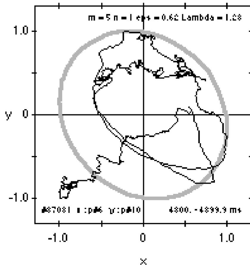
**Fig. 14** Lissajous diagrams of a pair of Mirnov signals ( $\delta B_1$  vs.  $\delta B_2$ ) show strongly distorted space coherence.
