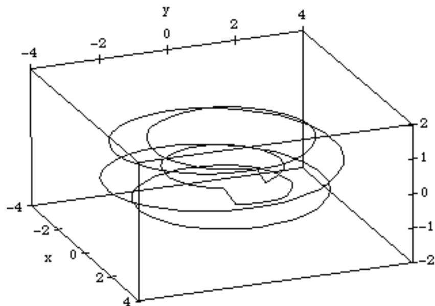
**Fig. 7** Halo currents that are interrupted by structures are discrete and incompletely helical ‘bundles.’
