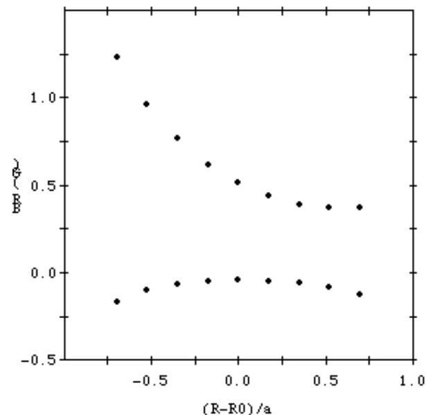
**Fig. 8** ‘Interrupted’ halo currents produce much greater  $B_r$  (top ‘curve’) than completed helical currents (bottom) for a unit current (1 kA).
