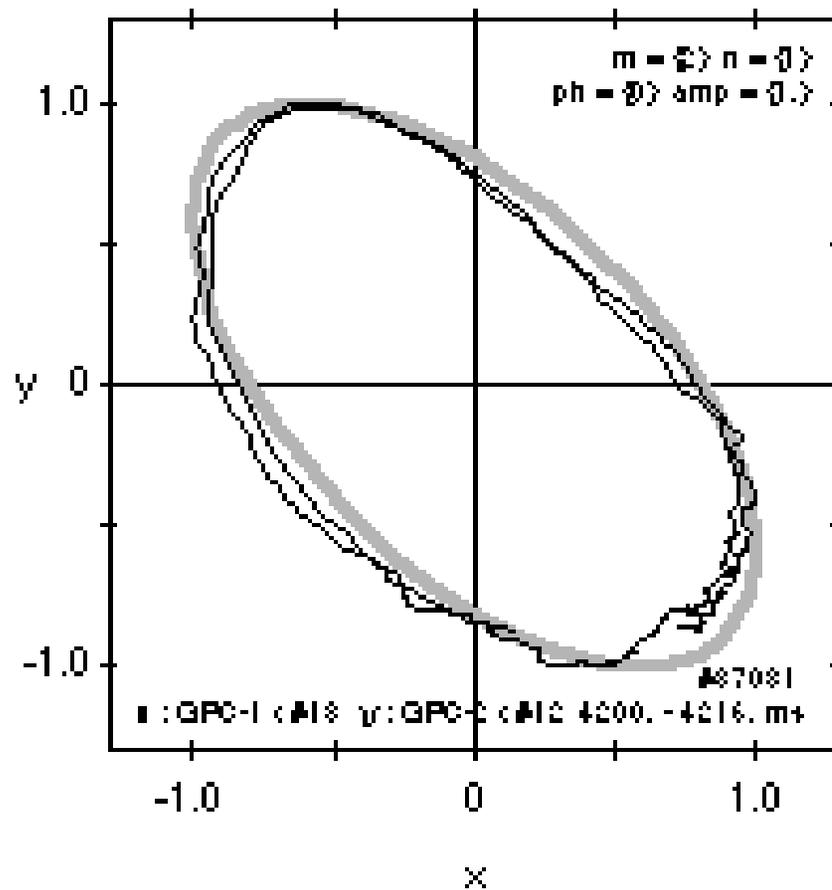
**Fig. 18** Lissajous diagrams of a pair of  $T_e$  perturbation signals ( $\delta T_{e1}$  vs.  $\delta T_{e2}$ ) 'just before locking time' — still good space coherence *unlike* external magnetic signals.
