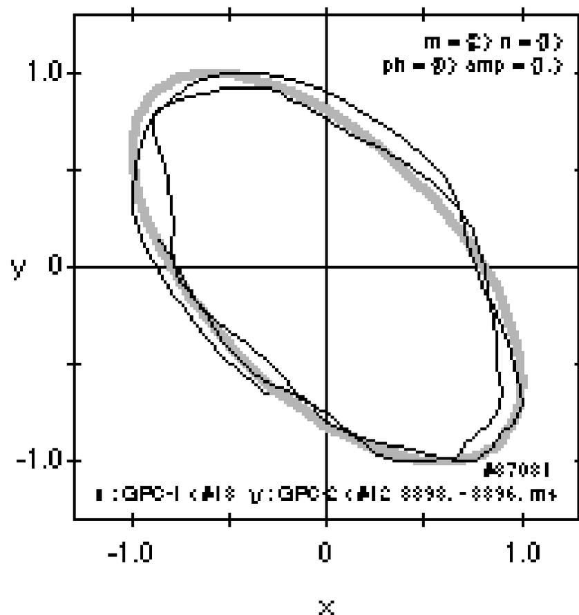
**Fig. 17** Lissajous diagrams of a pair of  $T_e$  perturbation signals ( $\delta T_{e1}$  vs.  $\delta T_{e2}$ ) 'well before locking time' — good space coherence.
