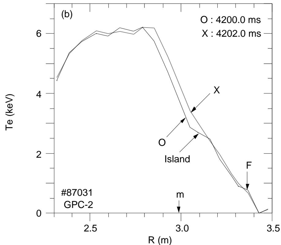
**Fig. 15**  $T_e$  profiles from GPC-1 signals show an island structure ‘just before locking time.’
