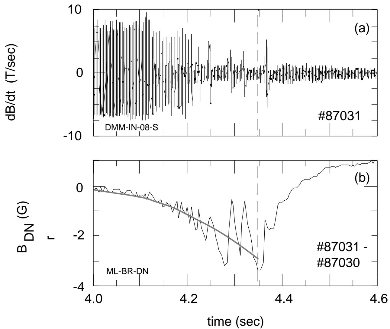
**Fig. 2** Mirnov coil and SMP sensor signals in an SMP event. (a) Oscillation frequency of Mirnov signal slows down. (b) SMP signal builds up *secularly* while *oscillating* at the same time. We call this type a 'compound' SMP for this reason.
