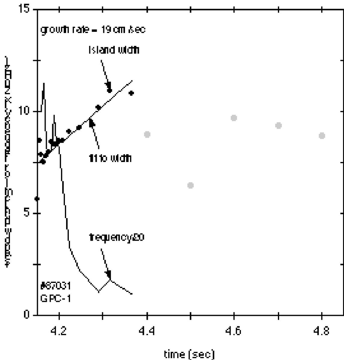
**Fig. 19** Island width and rotation frequency measured by ECE. Island is growing before ‘mode locking,’ with a growth rate that is little affected by mode slow down. Island does not grow after locking (points after locking in gray), contrary to a theoretical expectation.
