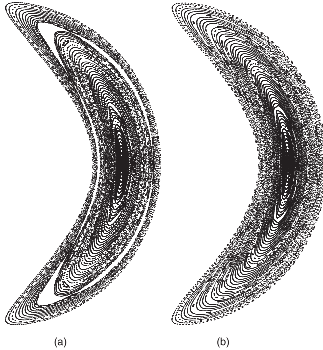
Figure 2. Poincaré plot of flux-surface structure: (a) original target plasma of figure 1, (b) with boundary perturbed to remove islands (fewer flux surfaces plotted).
