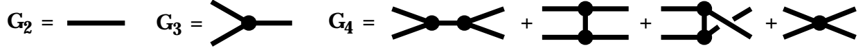
Fig. 19. Relationships between the first few cumulants and renormalized vertices. Successive diagrams follow by differentiation with respect to \eta_1 , using the rules that (i) the derivative of a line inserts a vertex, and (ii) the derivative of a vertex raises its order by one. The first term of G_4 is the DIA; the last three terms represent all of the doubly connected contributions omitted in the DIA.
