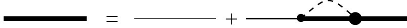
Fig. 10. The complete Dyson equation for R includes both propagator and vertex renormalization. R^{-1} = R_0^{-1} + \Sigma^{\text{nl}} , with \Sigma^{\text{nl}} = -\widehat{M}R\Upsilon R\Gamma .
