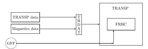
BRAZIL-1/frozen The TRANSP "Equilibrium Driver" phase , where FRBC input data is passed into what is a TRANSP shell, where everything but the equilibrium code is shut off. In this mode, the profile data that is input must conform to the profile data used by the FRBC codes in standalone. So, for VMEC, that means inputing pressure and magnetic field pitch angle as a function of major radius.
