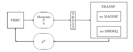
**BRAZIL-2** In the second phase the FRBC calculation is internal to TRANSP. The *input* data now consists of switches and magnetic coil and probe data. The pressure profile is developed internally, using the ususal TRANSP methodology.
