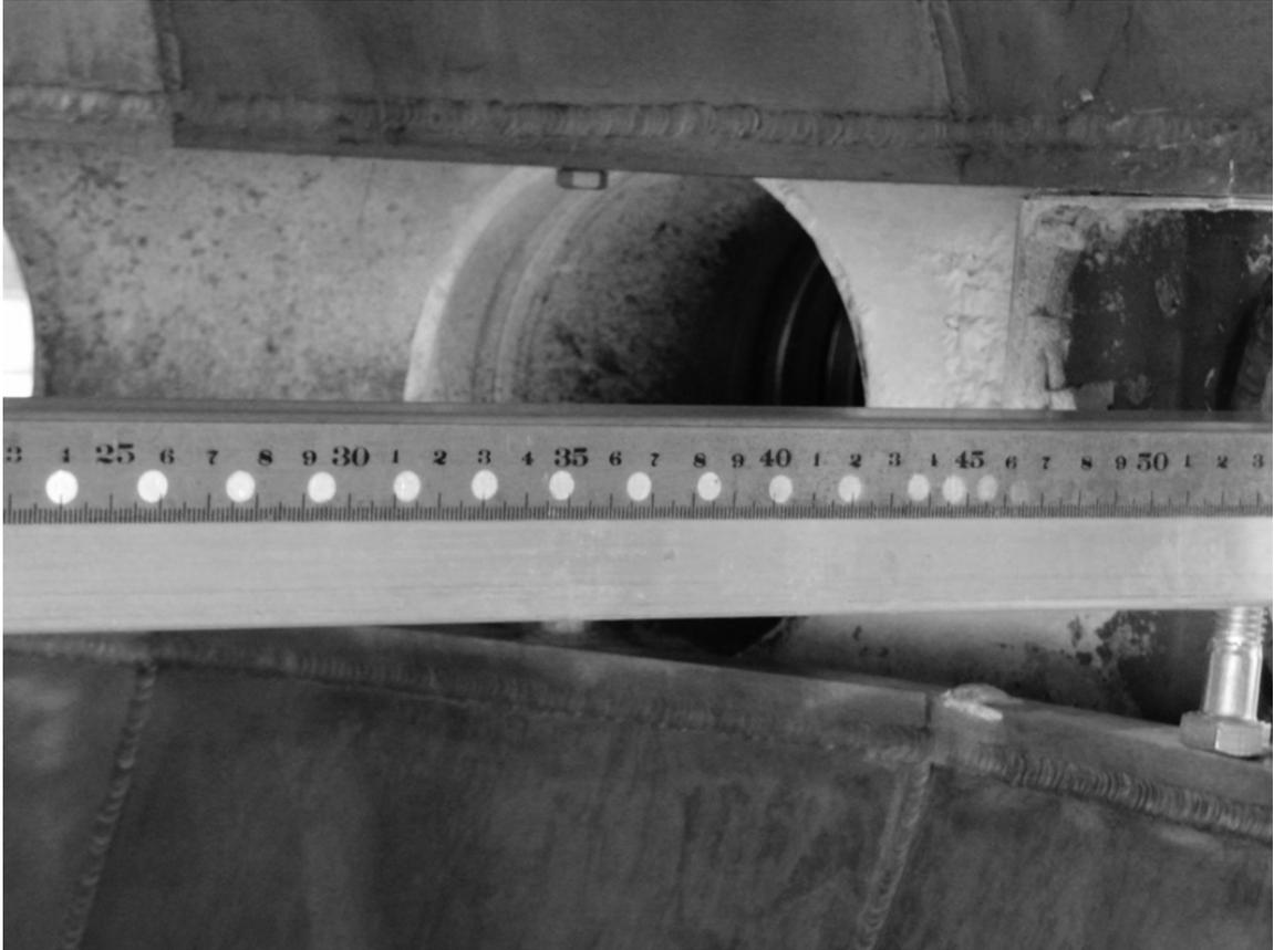
Figure 4.4: In vessel spatial calibration of toroidal views by illuminating fibers and photographing spots projected onto a ruler.
