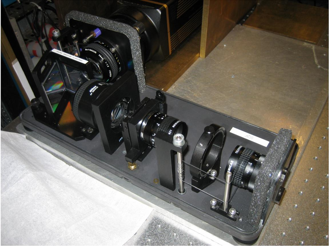
Figure 3.4: An image of the interior of the spectrometer. A metal cover has been removed for the photo. The fiber holder is normally connected to the right side of the spectrometer. Figure and caption reproduced from [45].
