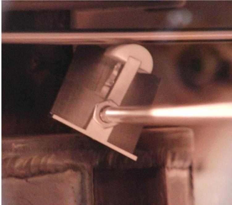
Figure 3.6: Re-alignment target assembly installed on vessel (top), and support rod on shell (bottom).
