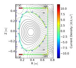
FIG. 5. Poloidal flux contours and toroidal eddy currents (shaded regions) from equilibrium reconstruction of LTX discharge 1504291321 at 474 ms. The location of magnetic diagnostics used in the reconstruction, flux loops (blue circles) and local field probes (blue crosses), are also shown.
