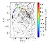
FIG. 3. Toroidal current source and corresponding poloidal flux contours for the upper shell segments created by toroidally averaging figure 2. The current source is shown with the same amplitude (but with a different color scale) as in the equilibrium given in figure 5, which corresponds to approximately 6 kA of circulating current in each of the upper shell segments.
