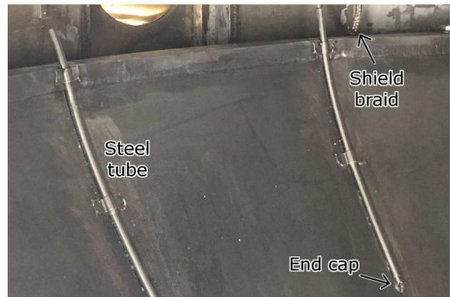
FIG. 3. The “In-Shell Sensors”, a set of three toroidally-discrete poloidal arrays of 10 sensors each, able to distinguish  $n = 1$  and  $n = 2$  structures. The tubes were infiltrated by creeping liquid lithium, disabling the Mirnov coils.
