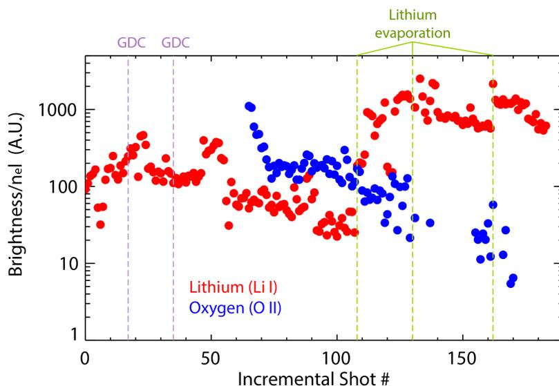
Figure 9. Lithium and oxygen levels, averaged over the early phase of the discharge (452 – 458 msec in Figure 5), for the recent dataset of discharges.
