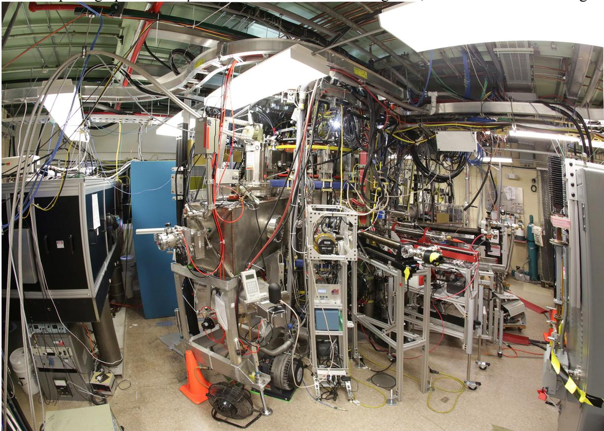
Figure 1. View of LTX- $\beta$  from the north. The main pump duct and the Thomson scattering laser (black enclosure) are to the left, in this view.
