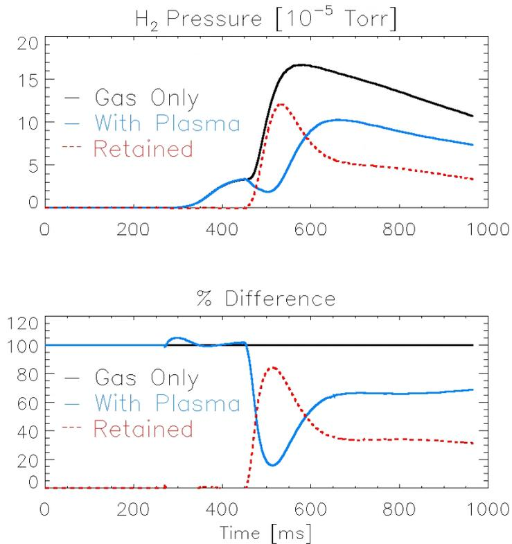
Figure 10. Torus gas pressure with and without a plasma discharge. About 1/3 of the total injected gas is retained long-term in the lithium wall. Although retention is significant, more analysis is required to derive a true recycling coefficient during the discharge.
