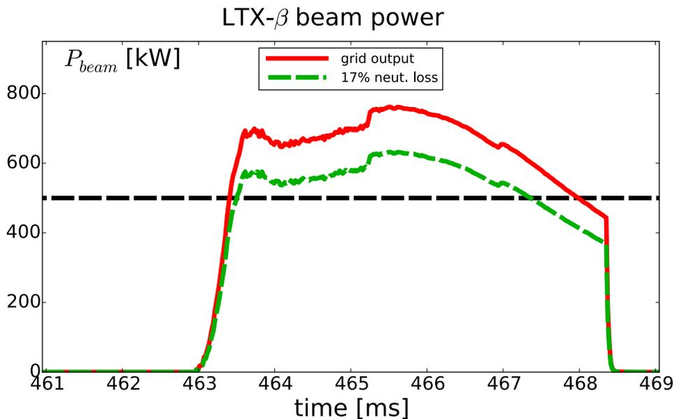
Figure 3. Ion (red) and neutral beam power (green) during a 3 kG LTX- $\beta$  discharge.
