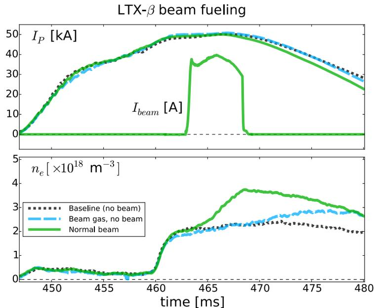
Figure 5. Comparison of the density rise in the discharge with beam injection (green line), and without beam (blue line). The neutral beam gas injectors were enabled for the “blue” discharge. Compared to a discharge without any beam gas, the blue “no beam” discharge shows evidence for modest gas fueling by the beam system, at late times. Beam injection provides a prompt, nearly linear rise in density.
