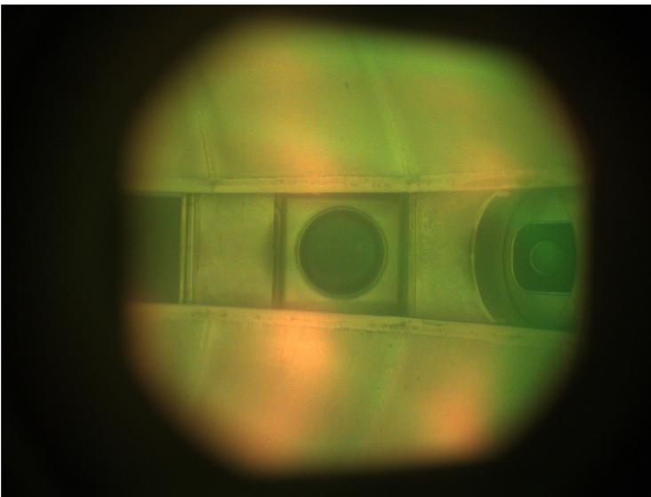
Figure 7. Fast camera image of the outer shell during a discharge. The green light is from the Lithium II line at 548.5 nm, while the yellow/orange light is from the Lithium I line at 610 nm.
