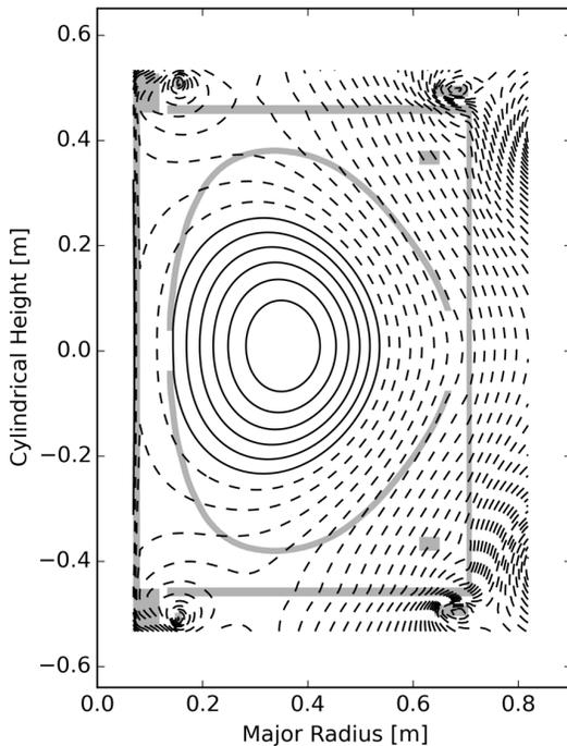
Figure 8. Equilibrium reconstruction of an LTX- $\beta$  discharge during neutral beam injection, with full lithium coatings, at 3 kG toroidal field. The current centroid is at  $R=31$  cm ( $B_{TF} = 3.5$  kG), and the Shafranov-shifted magnetic axis is at  $R=35$  cm ( $B_{TF} = 3.1$  kG). Plasma elongation is low ( $\kappa = 1.3$ ), but discharge development is ongoing.
