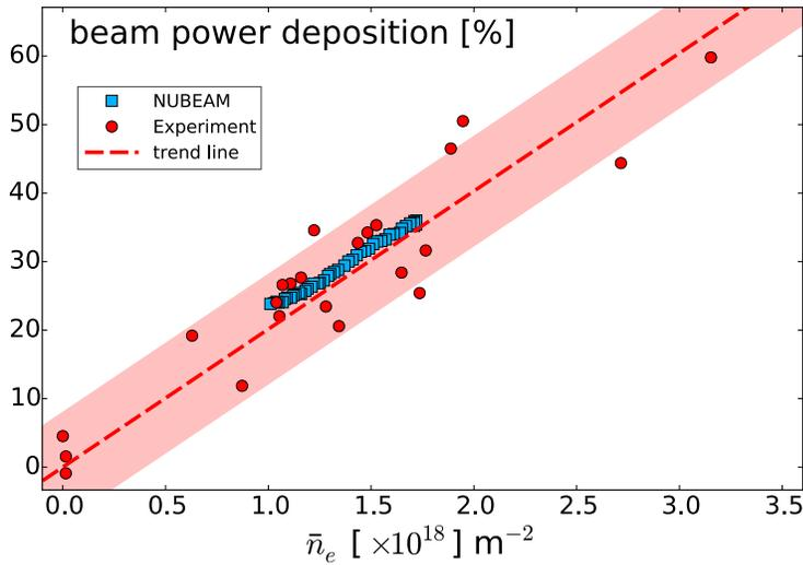
Figure 4. Measured and calculated (with NUBEAM) beam power deposition in the LTX-β discharge. The red dashed line is a fit to the experimental data.
