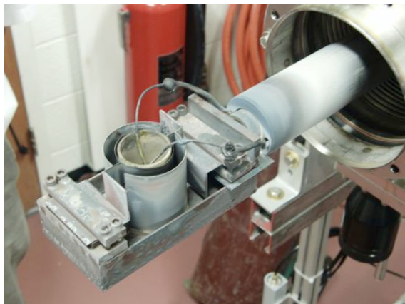
Figure 1. One of the LTX evaporator crucibles after initial use. 2 evaporators, 180° apart toroidally, are installed. Each crucible is typically filled with 8 grams of lithium. Typically a total of 4 grams of lithium is used per evaporation. The crucibles are ceramic yttria, and are not attacked by liquid lithium at temperatures up to 600 °C.
