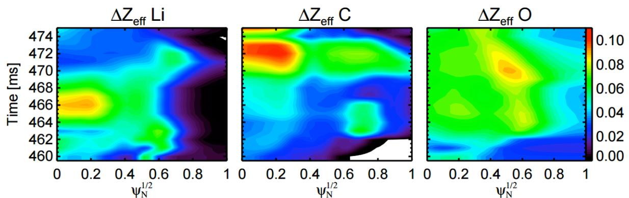
FIGURE 2. Contour plots of the evolution of the contribution of lithium, carbon, and oxygen to the discharge  $Z_{\text{effective}}$  in LTX. Carbon and oxygen are the primary impurities in the discharge.
