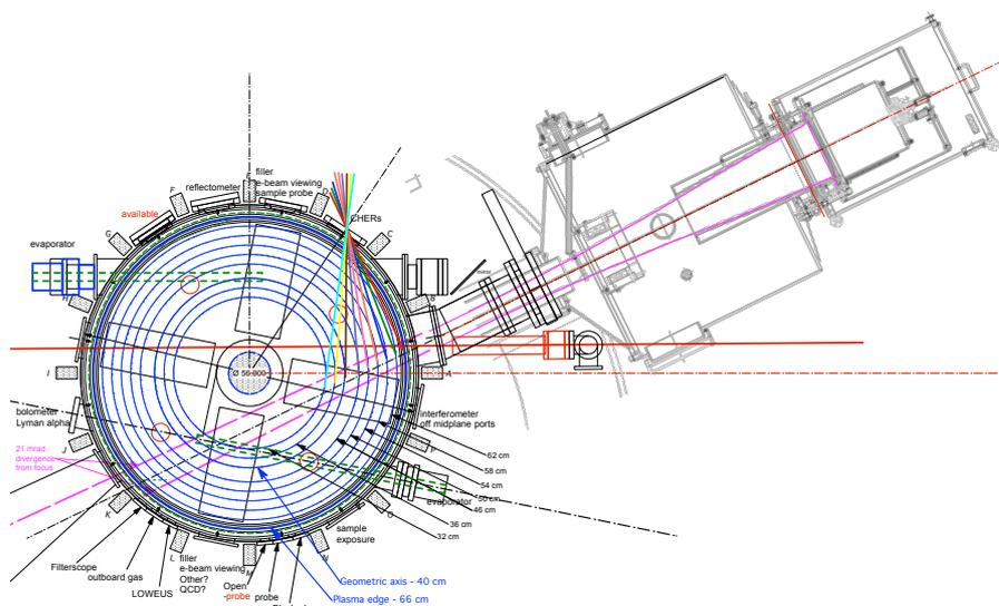
FIGURE 5. Layout of the neutral beam installation on LTX.
