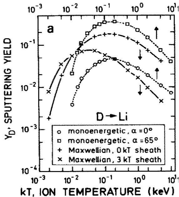
FIGURE 3. TRIM-SP calculations of the sputtering yield for deuteron impact on lithium, from Laszlo and Eckstein, 1991. The various curves are calculated for different sheath conditions and ion energy distributions. All the sputtering yields peak below 1 keV.
