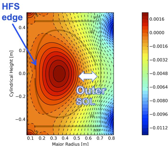
FIGURE 4. Equilibrium reconstruction of the LTX plasma with the PSIOTRI code (U. Washington). The distance between the outer LCFS and the shell-defined wall is 10 - 12 cm at times when the electron temperature profile is fully flat.
