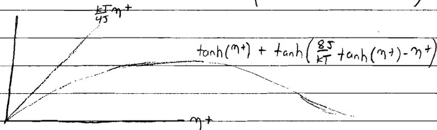
Below  $T = T_c$ , Ferromagnetic behavior occurs where there is a nonzero possible value for  $\eta^+$  (and hence  $\bar{S}_{+z} + \bar{S}_{-z}$ ) at zero applied field.
