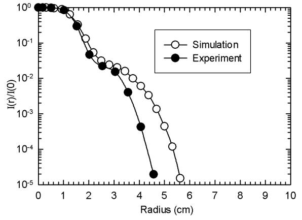
"Simulation" is a 3D WARP simulation that includes injection from the ion source.
