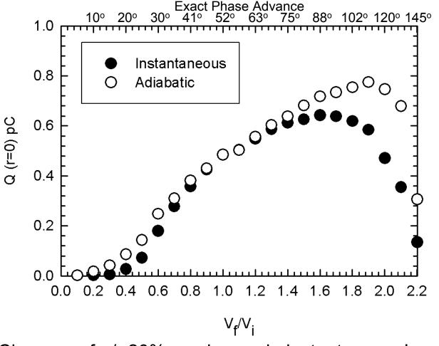
Adiabatic means 40 lattice periods for 90% of the hyperbolic tangent transition from V<sub>i</sub> to V<sub>f</sub>.
