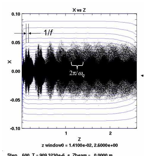
Oscillations can be seen at both f and the  $\omega_q$  near z = 0.
