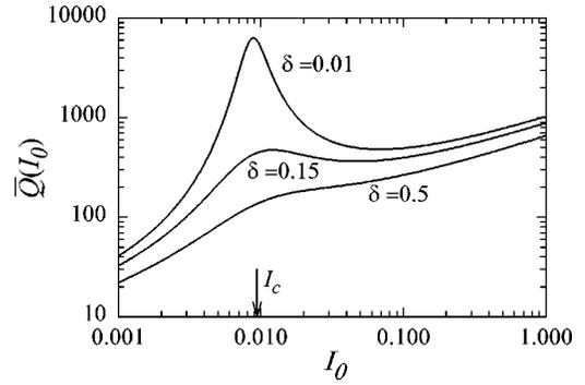
FIG. 1. The function  $\bar{Q}(I_0)$  defined by Eq. (15). The system's  $Q$  must exceed this function for the pseudopotential wells to exist and for the system to stay in autoresonance.  $\bar{Q}(I_0)$  is plotted as a function of  $I_0$  for three values of drive strength  $\epsilon = (1 + \delta)\epsilon_c$ . The arrow marks the critical action for  $\delta = 0$ , and  $\beta = 0.6$ .
