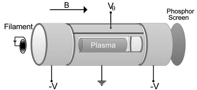
FIG. 2. Basic trap geometry. The plasma is emitted from the filament, and loaded into the trap by temporarily grounding the left cylinder. Details of the trap operation can be found in Ref. 18.
