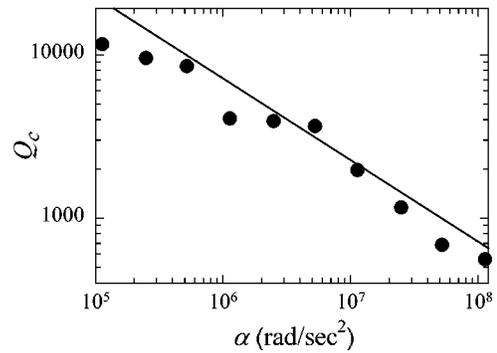
FIG. 6. The measured minimum autoresonant  $Q_c$  as a function of the sweep rate  $\alpha$ , for  $\delta = 0.03$ . The results (circles) are compared to the prediction (line) of Eq. (17); there are no adjustable parameters. Note that  $Q_c \propto 1/\sqrt{\alpha}$ . The parameter  $\delta$  is relative to the measured  $\epsilon_c$ .
