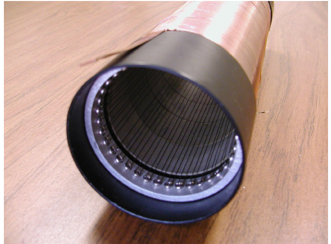
Fig. 1. Photograph of the 20 cm-long PZT ferroelectric source.
