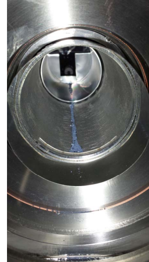
Fig. 9. Lithium granules (gray spheres) on the bottom of the injection baffle, and TIV copper seal and valve bottom.
