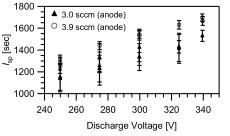
Fig. 5  $I_{sp}$  as a function of discharge voltage. The error bars represent a 95% (2 $\sigma$ ) confidence interval.
