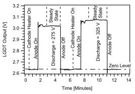
Fig. 3 Raw LGDT output data as a function of elapsed time for two thruster operating points.
