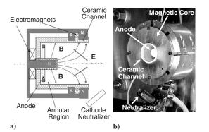
Fig. 1 PPPL cylindrical Hall thruster: a) schematic illustration and b) photograph.
