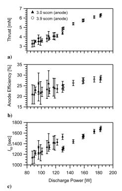
Fig. 4 Performance measurements for a 3-cm cylindrical Hall thruster: a) thrust, b) anode efficiency, and c)  $I_{sp}$  as a function of discharge power. The error bars represent a 95% ( $2\sigma$ ) confidence interval.
