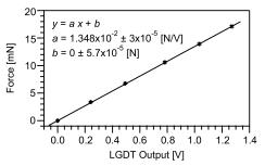
Fig. 2 Applied calibration force plotted as a function of LGDT response. The linear curve is a fit to the displayed data. Error bars on the data points and the fit coefficients represent a 68% ( $1\sigma$ ) confidence interval.
